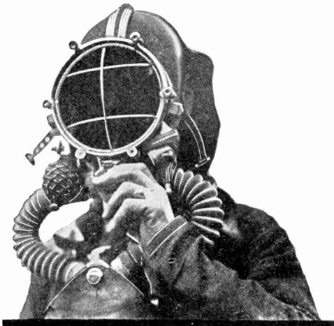
OXYGEN HELMET IN WHICH THERE IS ALSO ENCLOSED A TELEPHONE
