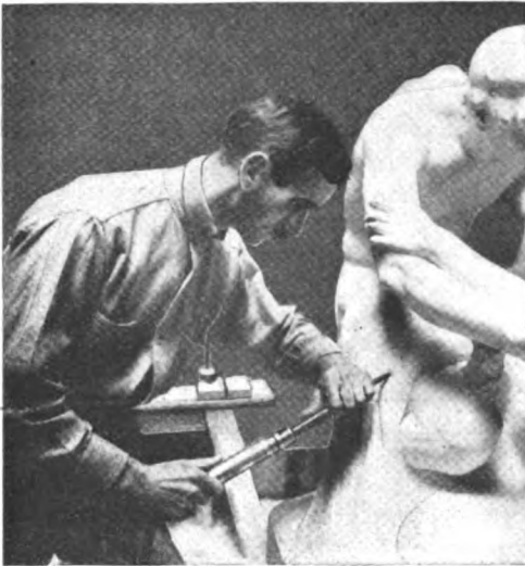
Roughing Out the Marble by Means of an Electro-pneumatic Chisel
