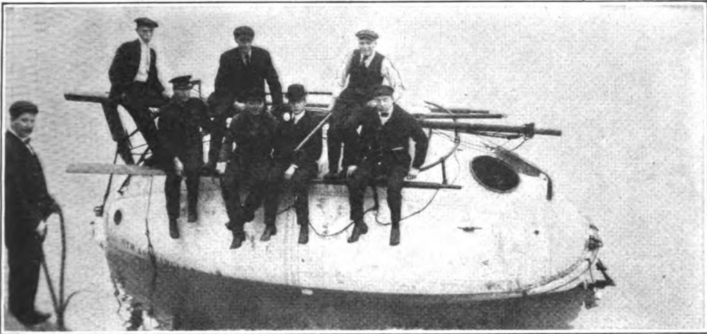
There Is Room to Seat 33 People Inside the Brude Boat and Several More Can Cling to the Outside
