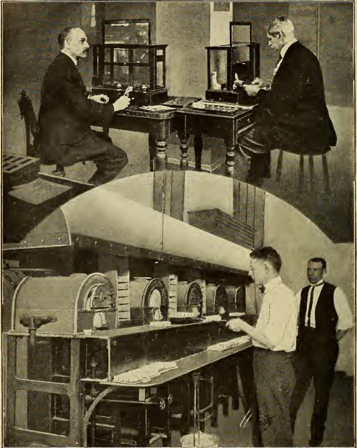
THE DELICATE SCALES OF THE ASSAYER'S OFFICE FURNACES FOR HEATING TINY CRUCIBLES
