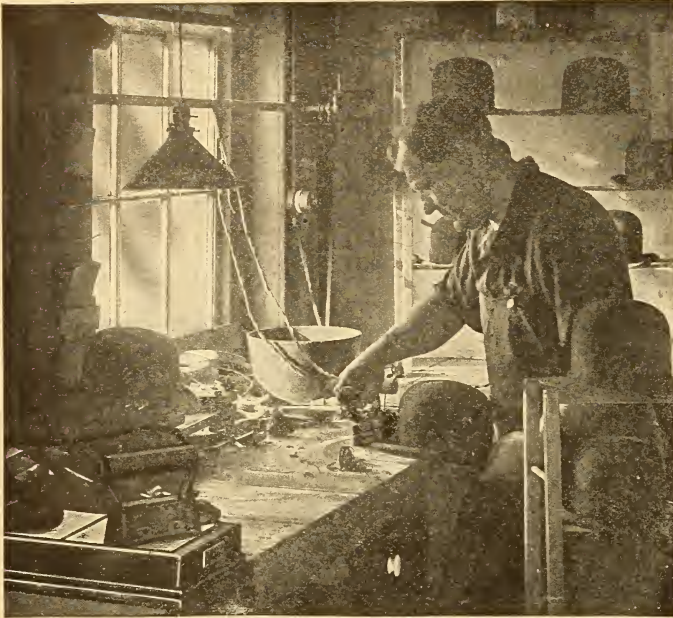
USING THE "SHACKLE IRON" TO CURVE THE BRIM
