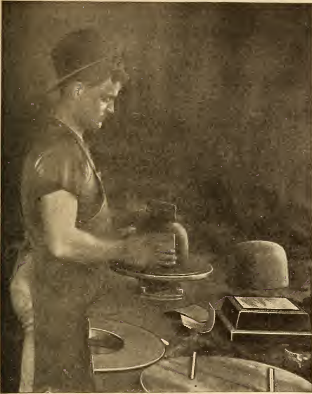
THE "LURING OFF" PROCESS, SHOWING THE ELECTRICAL VELOURING STOVE
