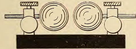
FIG. 1. SPARK GAP FOR SMALL UN-TUNED TRANSMITTER
