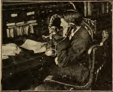
Permits one to adjust telephone to their position, not adjust self to position and convenience of telephone
