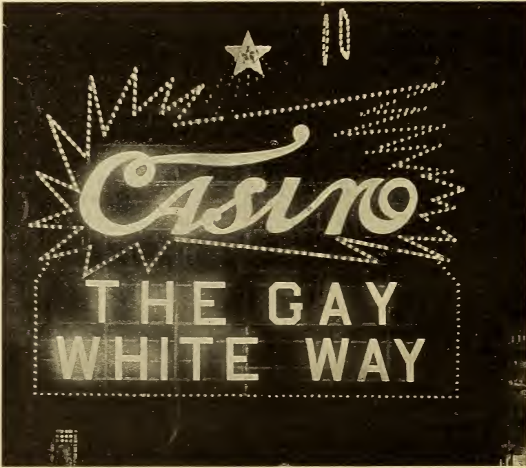
FIG. 1. SIGN REQUIRING THE COMBINATION OF FIVE FLASHERS.
