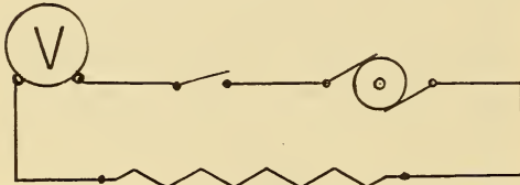
FIG. 1. VOLTMETER METHOD OF DETERMINING RESISTANCE.
