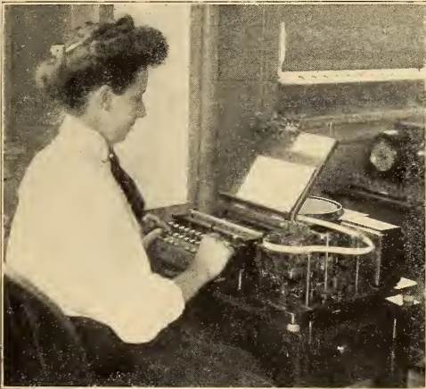
Copyright, 1908, by J. R. Schmidt, Cincinnati, O. FIG. 1. PUNCHING TAPE FOR PRINTING TELEGRAPH.
