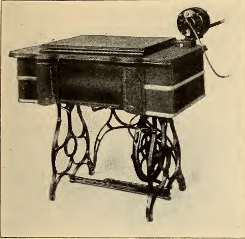
MOTOR APPLIED TO DROP-HEAD SEWING MACHINE.
