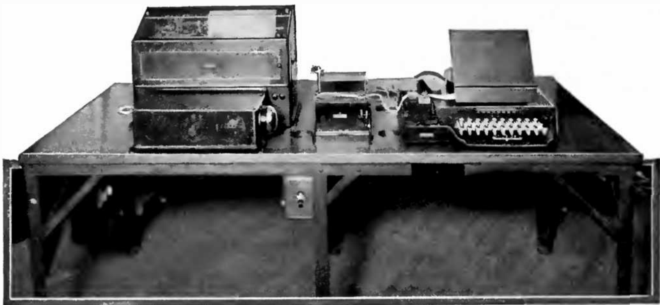
A Multiplex Table Equipment of the Printing Telegraph. On the Left is Shown the Printer with its Relay Box, the Transmitter and Automatic Control are in the Center, and on the Right is the Keyboard Perforator. Four of these Table Equipments would be Required at Each End of the Line in a Quadruple-Duplex Installation.
