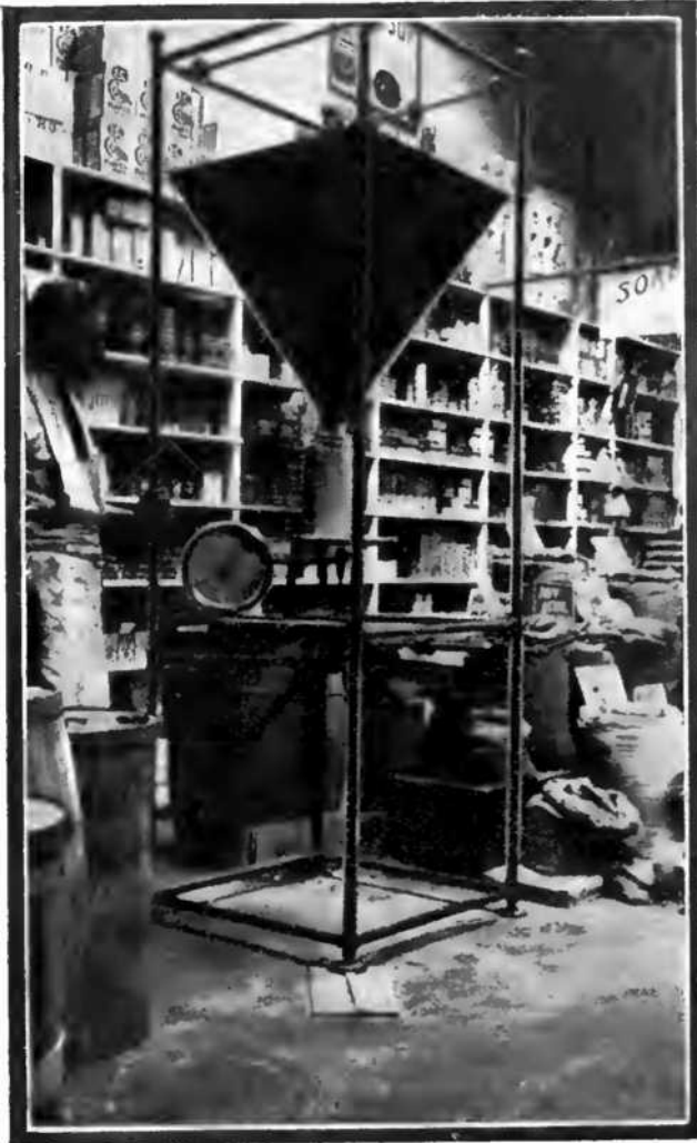
Much Time and Labor is Saved by the Use of the Electric Weigher, Which Automatically Weighs Out Goods in Bulk.
