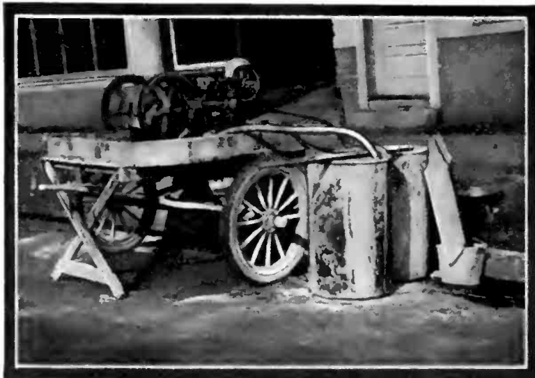
This Home-Made Machine Constitutes a Very Complete and Useful Paint Sprayer. As the Illustration Shows, it is Quite Portable and, Although Crude in Construction, the Device is Capable of Heavy and Practical Service.
