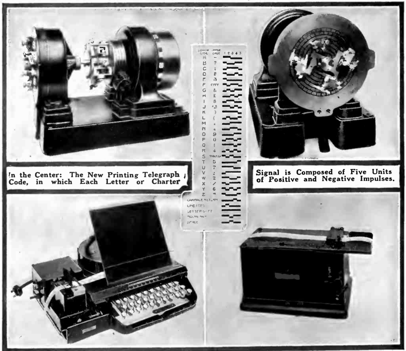
Above, to the Left: The Distributor Motor and Its Mechanical Corrector which Automatically Steps Back the Brushes at the Fast End when They Have Gained a Small Angle on the Brushes at the Slow End. To the Right: The Distributor by Means of Which Four Messages may be Sent Simultaneously. Below, to the Left: The Keyboard Perforator which Prepares the Tape for the Transmitter which is Shown at the Right.
