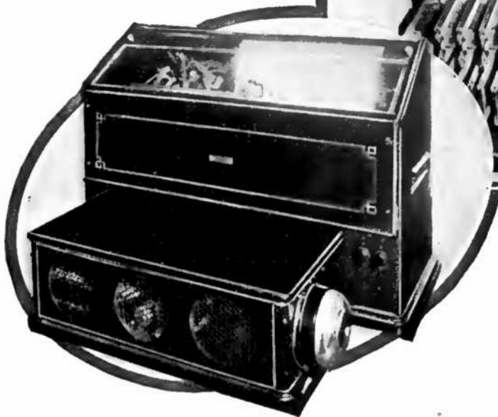
Interior and Exterior Views of the Printer and Relay Box. This Mechanism Receives the Impulses from the Sending End and Delivers the Message, Ready for Delivery to the Addressee, Neatly Printed in Type. A Novel Feature of the Mechanism is Its Unit Construction which Permits of the Removal of Any Separate Unit for Repairs without Dismantling the Entire Machine
