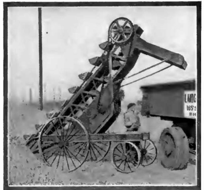
This Electrically-Driven Machine Takes the Place of Several Laborers in the Loading of Broken Stone, Sand, Gravel and Other Similar Material.
