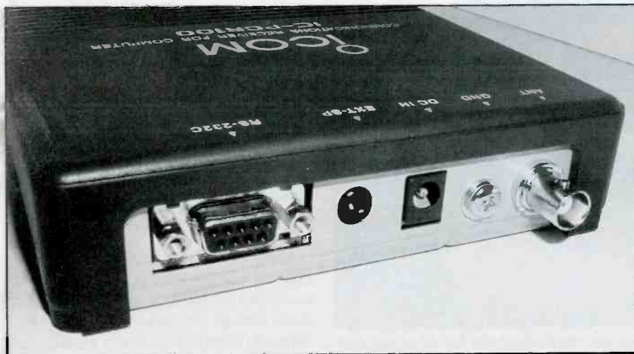
Receivers like this PCR-100 from ICOM require a computer to function. Just plug the supplied cable into the 9-pin connector at the left and away you go!
