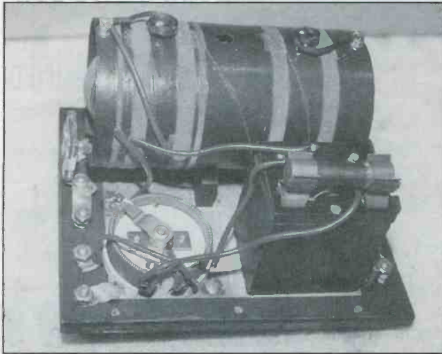
This inside view shows the large antenna coil at the top, and the filament rheostat at bottom left. The large black object is the tube well-and-socket assembly. The cylinder-like object that resembles a 30-amp fuse is a cartridge version of a combined grid leak resistor and capacitor.
