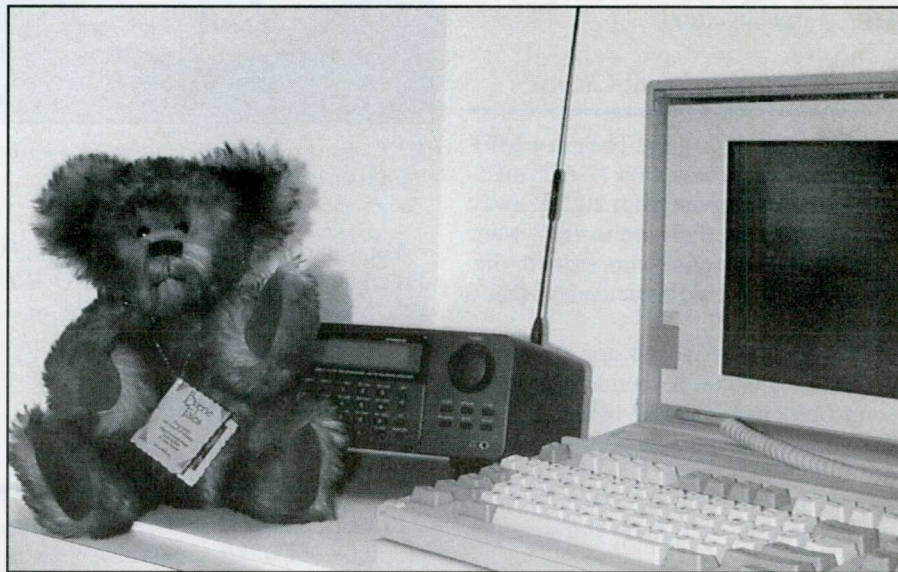
Bartholomew says "Hey folks, if I can figure this out, so can you!" An old IBM semi-portable and an Optoscan-controlled PRO-2042 make an excellent computer control system.
