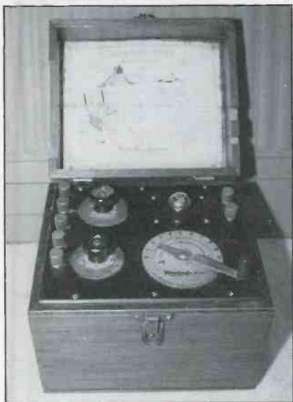
The Westinghouse Aeriola Sr. one-tube regenerative receiver. The top of the WD11 tube is just visible sitting in its recessed socket. At left, the top control sets the regen level, while beneath it is the rheostat. The large center dial is for tuning.
