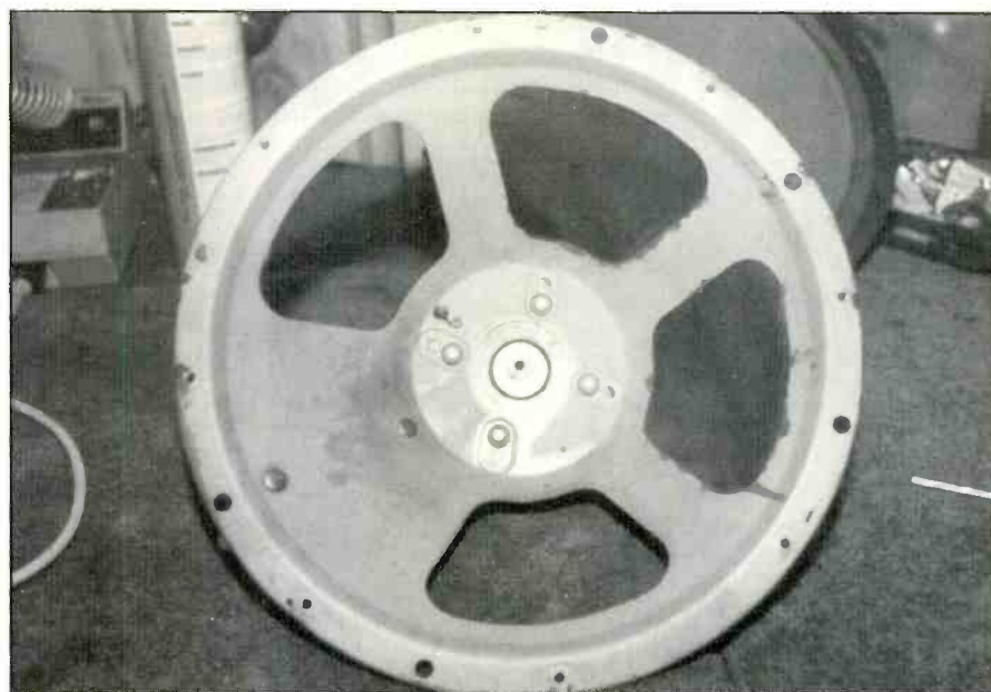
With the speaker cone removed, the magnetic pole piece the voice coil bobbin rides over is clearly seen. Note the very tight tolerances! The mounting hole for the spider lockscREW is easily seen in the center of the magnetic pole piece.
