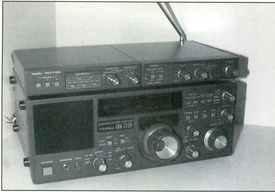
This is a complete receiving station made by Yaesu some time back, but it's still available on the used market. Note that active antenna visible on the right. With this system alone or another active antenna, you can spend many hours listening to shortwave.
