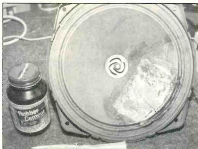
Generous applications of rubber cement are applied over the tear, and on the teabag paper used for a patch. This photo shows the cone and the suspension system between its outside circumference and the metal speaker frame.
