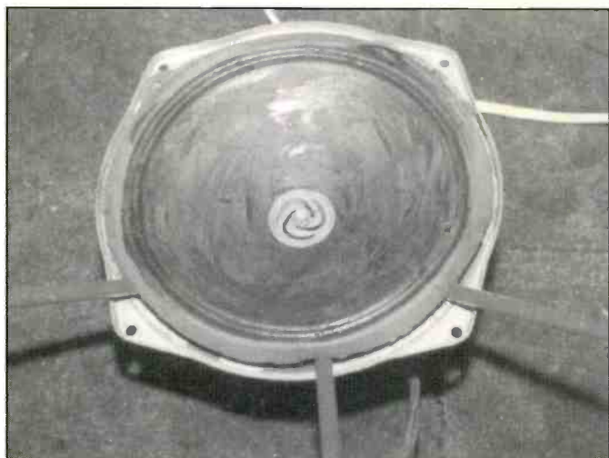
The adhesive between the speaker frame and the suspension of this speaker has failed, allowing the cone to separate from the frame. It needs to be reglued to prevent "rattles." This photo also gives a good view of the centering spider and its lockscREW.
