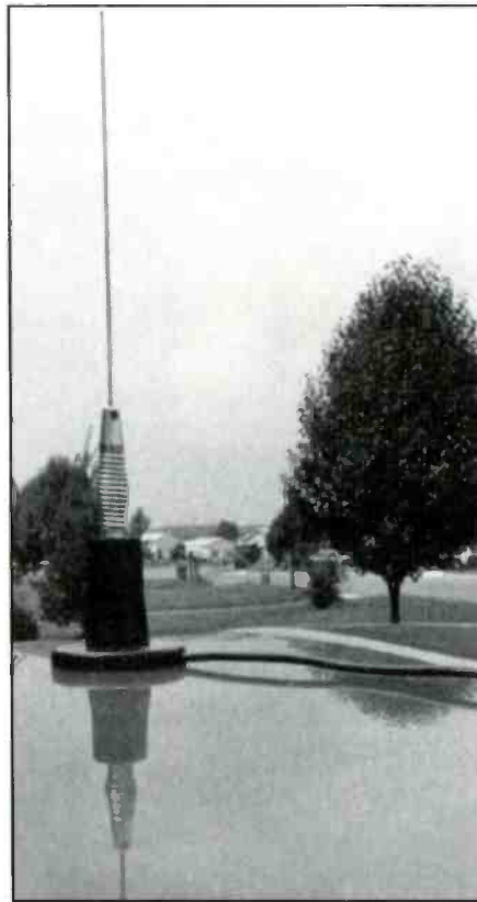
It may not be a full 102-inch fiberglass whip, but mounting your CB antenna in the center of your car's roof will give best all-around performance on transmit and receive.
