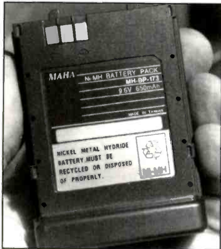
Nickel metal hydride batteries will play almost twice as long as NiCds, but require careful charging!
