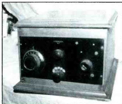
Photo A: Exterior view of the Crosley 1924 battery set. Cabinet was large enough to hold batteries.
