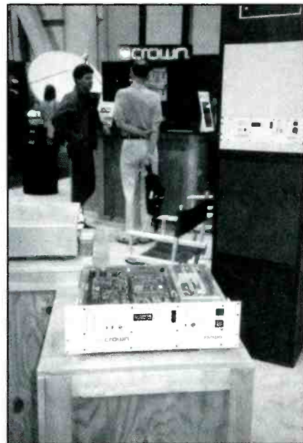
Dial in a good frequency between 88-108 MHz, plug in a mic and consumer-grade portable CB player into one side of Crown's 100 watt FM broadcast transmitter and an antenna in the other. Next, add 12 volts of battery, solar or wind-generated power and you're on the air. Missionaries using these tiny "plug-n-play" FM stations in densely populated areas can send a signal to millions.
