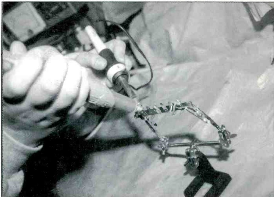
Photo C: My son, Tom helps to demonstrate the use of a solder sucker to remove excess solder from a terminal. This helps to find room when its time to add the replacement components leads. Ample heat is assured by the using the 33 watt Ungar soldering iron.
