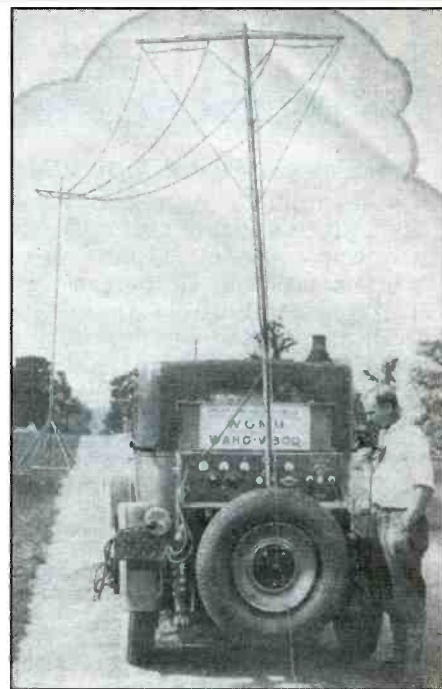
Portable broadcaster WGMU (with its call letter sign in the rear window) shown performing field-strength tests about 1931.
