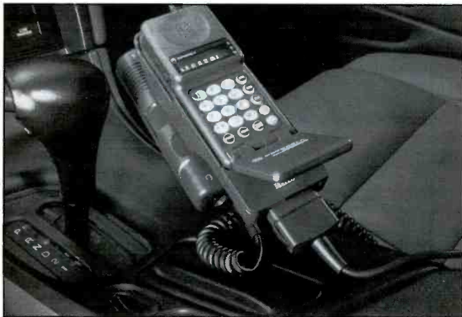
The universal car kit CellBase turns a handheld cellphone into a hands-free mobile phone.
