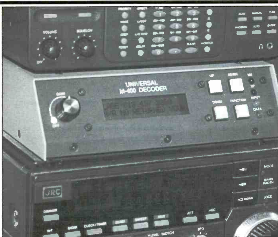
Universal's M-400 decoder tackles numerous tasks, including reading out CTCSS tones for you.
