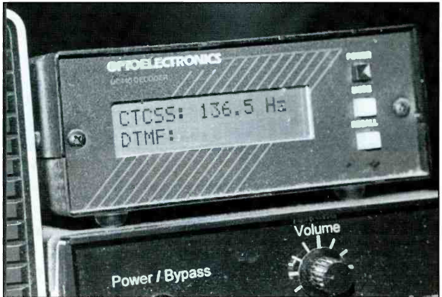
The Optoelectronics D440 decoder displays CTCSS tones to help you identify unknown stations. It also decodes DTMF tones.
