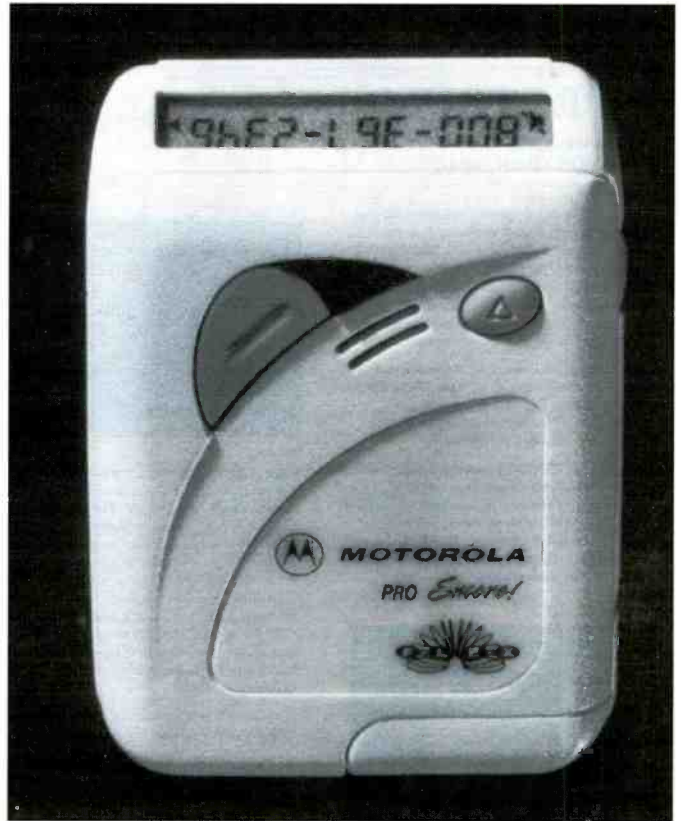
Motorola's Encore numeric pager operates in the new high-speed FLEX protocol.
