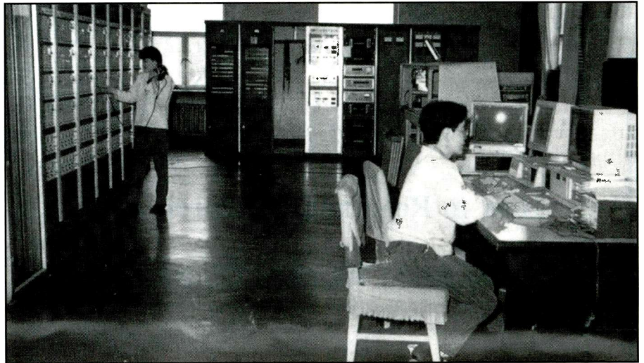
The control room at the main transmitter center of China Radio International. A computer distributes the 158 and a half daily broadcast hours in 38 foreign languages to the proper transmitter at the proper time.
