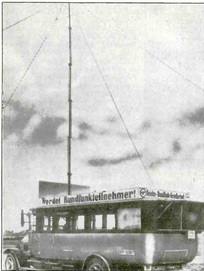
An early German mobile radio bus or van, showing a telescoping mast on its roof. (Courtesy Michael Schroter, Berlin Germany.)
