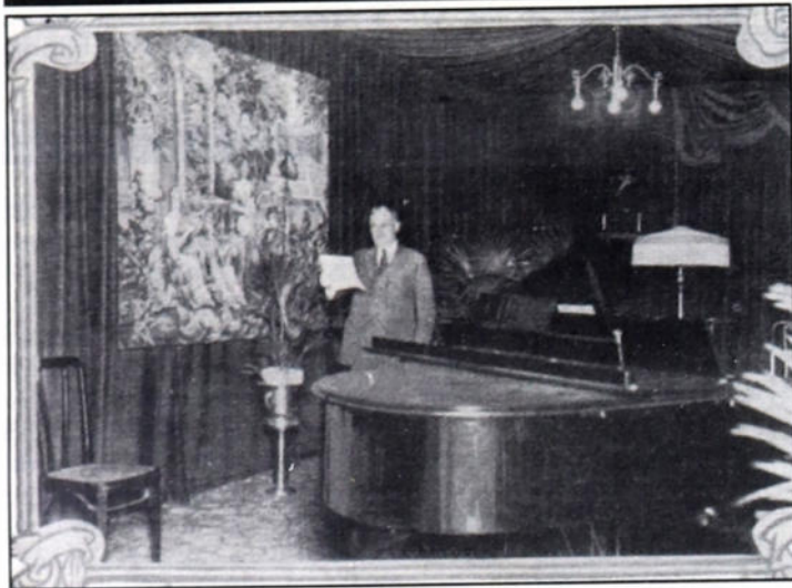
The luxurious WFBH studios were acoustically modified with carpeting, plus velvet covered walls and ceilings. Microphones were concealed to prevent "mic fright."
