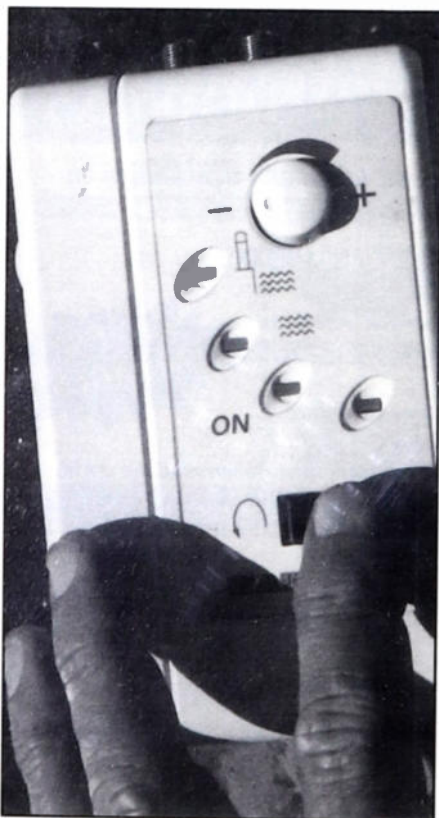
The rocker switch allows the beam to turn left or right for the best reception.
