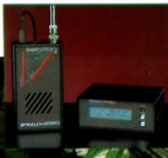
R10 checks coded squelch codes with DC440 Decoder
