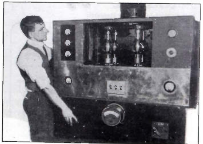
This was the 500 watt transmitter used by WFBH, which was the early version of WPCH.
