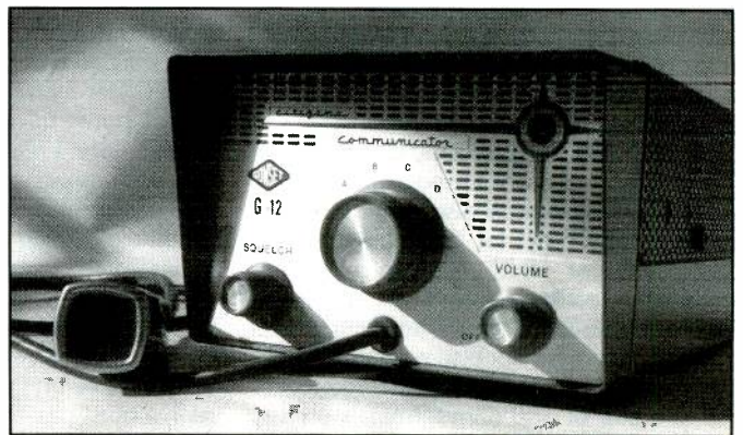
The Gonset G-12 had 4-channels and was a fine set, but wasn't glitzy enough to become a CB star. (Photo by D. Gillespie, Toledo, Ohio.)
