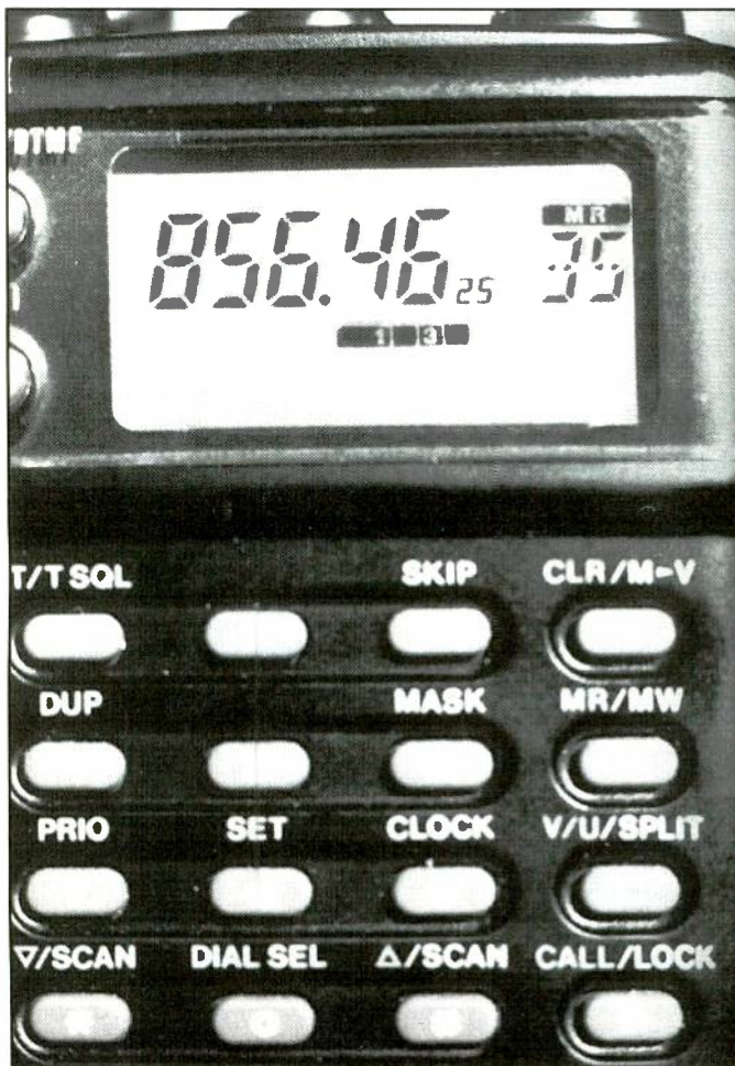
Some equipment will tune above 470 MHz plus go into 850 MHz on receive.
