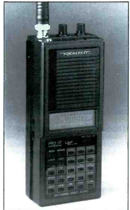
Realistic's PRO-37 is a hot 200-channel handheld scanner with "Hyperscan," plus 800 MHz coverage.
