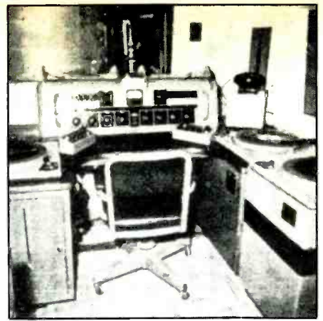
The VOWR control room looked like this in 1963. The hardware was mostly from Gates, with two Ampex 351 tape units and a National NC-109 receiver. (Courtesy Howard Kemp.)
