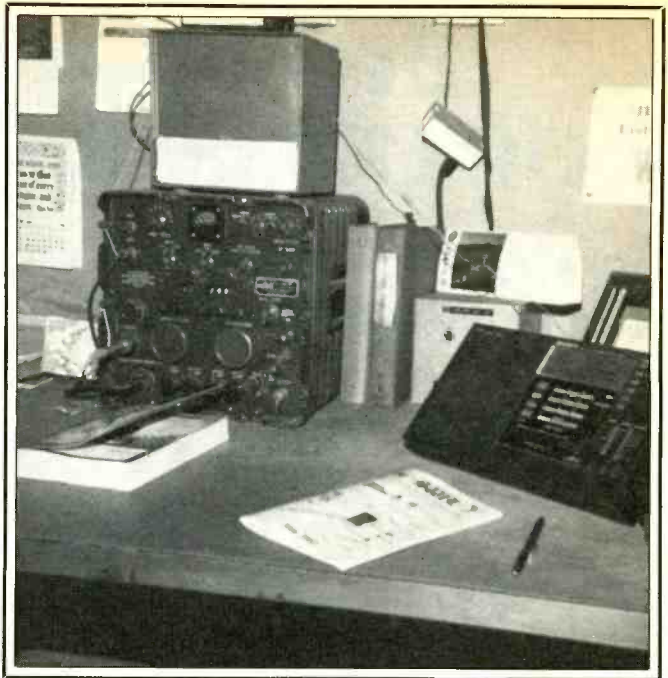
Listening post at ASWLC HQ's, consisting of a Collins R-392 (left) and a SONY 2001. Paperwork on the desk looks to be a copy of the WRTH and the ASWLC's own monthly publication, "SWL."
