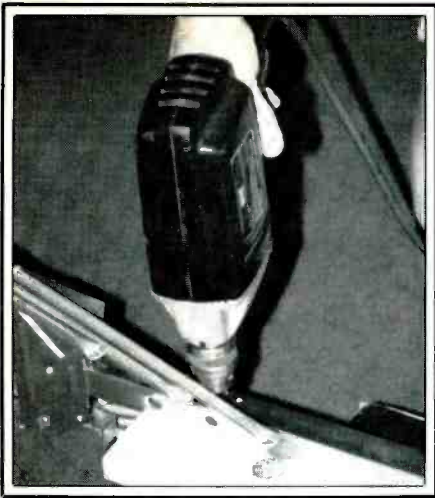
Modifying the antenna for receiving vertically polarized signals was simple. Drilling through the aluminum took only a few seconds.
