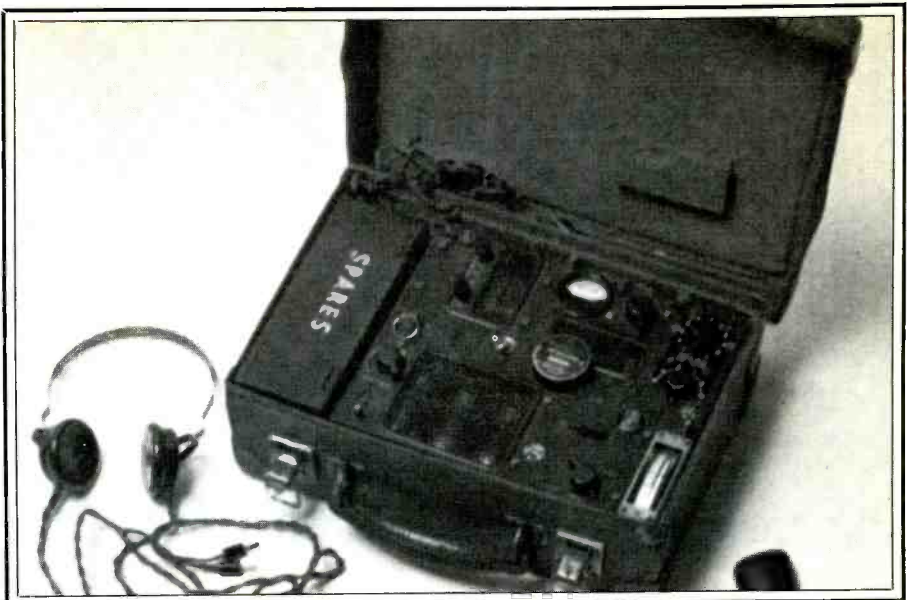
One of our readers provided the operating specs for this WWII spy transceiver. Says it ran 5 watts and had a 500 mile range!
