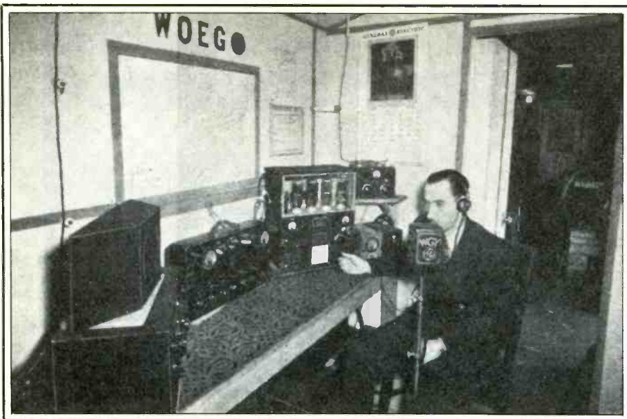
Station WOEG operated on 2000 kHz from a Union Pacific train in 1939. G.E. radio engineer, Bob Lingle, on loan from station WGY, is shown at the controls.
