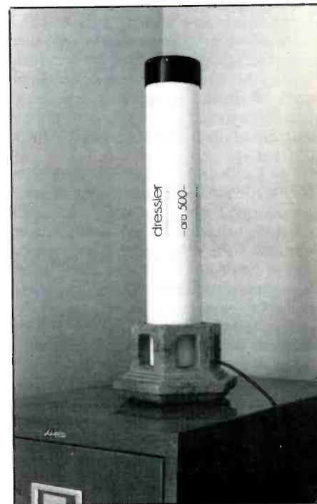
Fig. 2. Convenient indoor mounting of active antenna atop filing cabinet using a ceramic piece for support.
