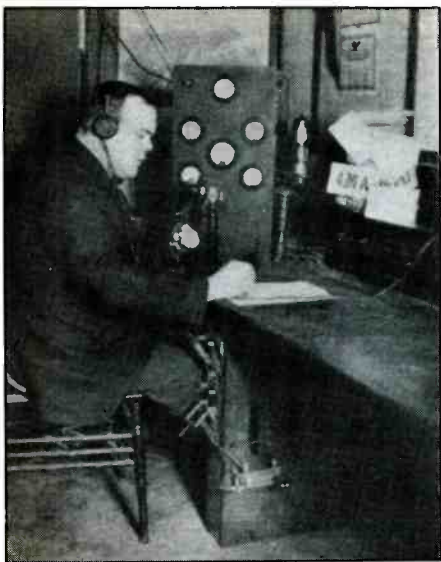
Harry Carman's ham station, 2EL (shown here in 1924) evolved into local broadcaster WGBB. Harry said the call letters meant "Where Good Broadcasting Begins." The rig shown here ran 50 watts. Receiver was a Grebe. At the end of January this year, WGBB sadly faded into history after 63 years of operation.
