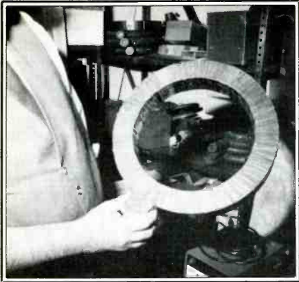
Mansbach shows off an old df loop antenna.
