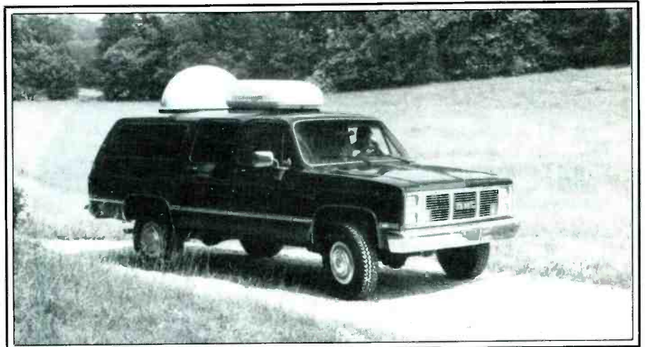
The VCS-9100 Vehicular Communications system. The dome at the rear of the vehicle houses the antenna. The pod over the cab is the air conditioner.
