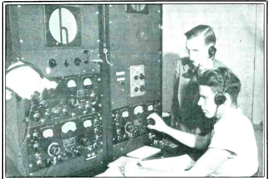
American radio networks carefully monitored the exact wording used by their overseas reporters in their stories. Even the informal chatter the technicians exchanged with the correspondents before and after the news reports often concealed carefully hidden information! This monitoring installation used two Hallicrafters SX-28 receivers operated by two fellows paying close attention to the traffic.
