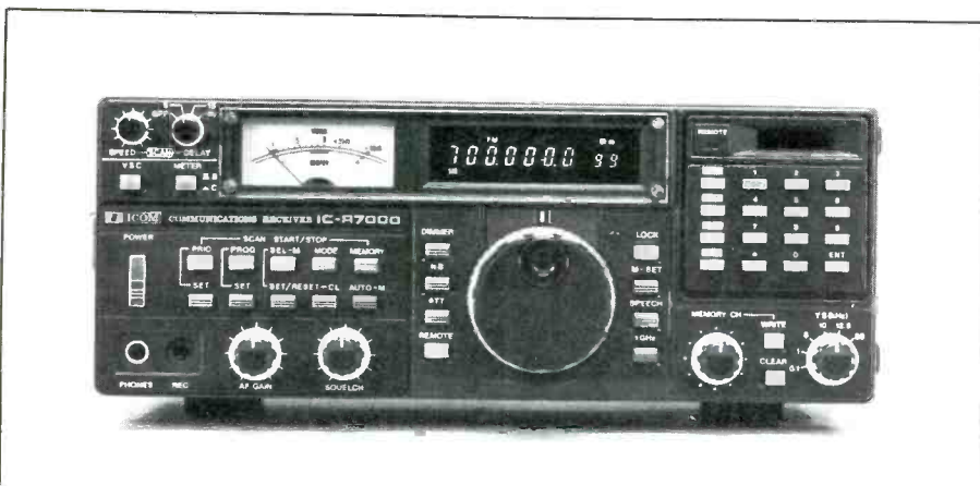
The ICOM R7000 scanner has the ability to continuously tune from 25 MHz to more than 2000 MHz.
