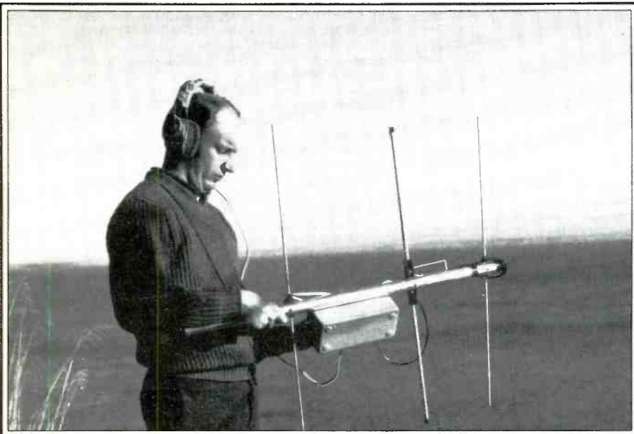
A portable shortwave receiver used for tracking purposes. (Photo by Matthew Perry)
