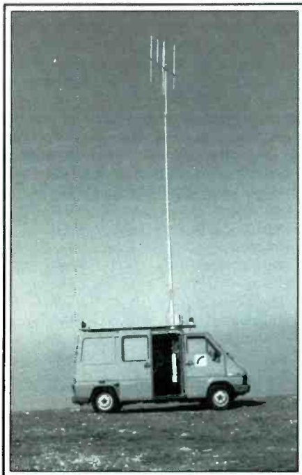
This Post Office relay van sports a hydraulic mast for ease in relaying broadcast signals.
