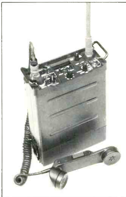
The AN/PRC-117 has a built-in scrambler.
