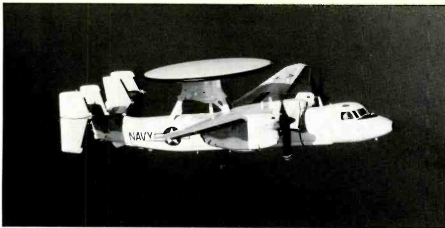
The Grumman E2C Hawkeye can track more than 250 radar targets from 250 miles out and then radio the information to ships and fighter aircraft. (Courtesy Grumman)
