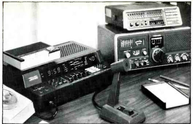
Survival communications here includes a scanner, a communications receiver, and an SSB base station.
