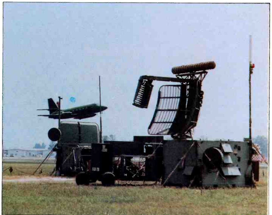
Portable air traffic control stations can be set up in almost any location to communicate with aircraft carrying advanced electronics devices. (USAF photo)
