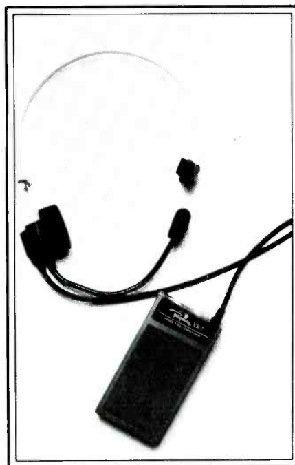
The Regency VX-7 is a precision short range communications device that operates in the 49 MHz license-free band. This makes it worthy of serious consideration for those who are wrestling with the dilemma of obtaining a license.
