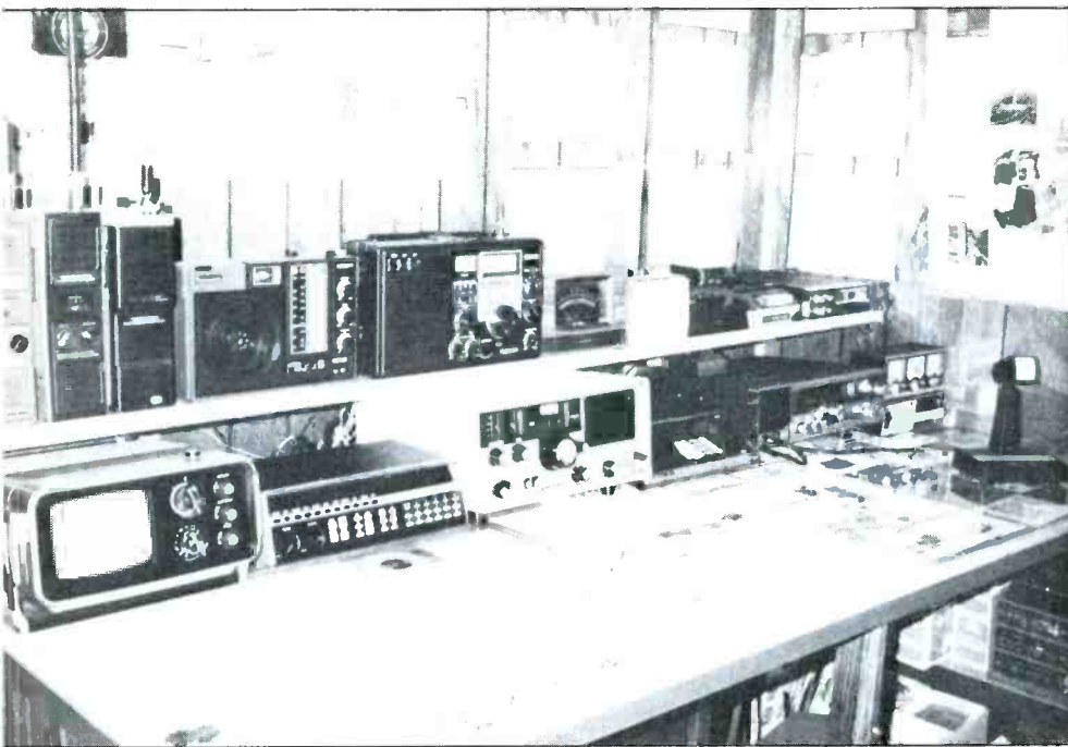
Here's the station operated by Denis E. Wilson, KNY2JS, of Gloversville, NY. Note the well organized layout. It's a simple task to run a grounding strap between all the pieces of equipment of a station such as this.
