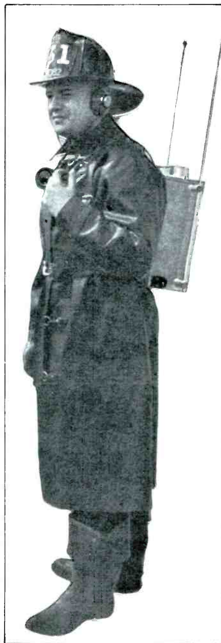
A 1930s NYFD fireman wearing backpack radio. Note the microphone and switch cable attached to harness straps.
