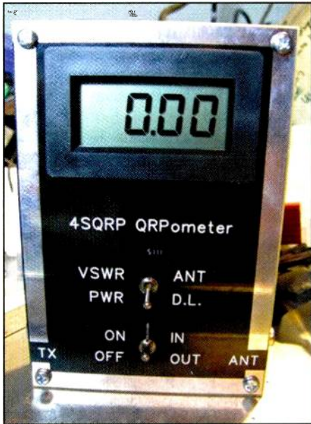
Photos B and C. To get the most out of low-power operating you have to accurately measure your power output, no matter how low it may be. Conventional power meters do fine from 50 to 1,500 watts, but it takes a true QRP power meter like the QRPometer shown here to achieve high accuracy between 1 and 10 watt. Designed by David Cripe, NMØS, and offered in kit form from 4SQRP (The Four State QRP Group), the QRPometer is an affordable, yet highly accurate, power and SWR meter that covers 100 mW to 10 watts. Designed for easy assembly, the kit uses all through-hole parts and requires no toroids. ( DETAILS: Visit < http://www.4sqr.com >.) (Courtesy of KØNEB and 4SQRP)
