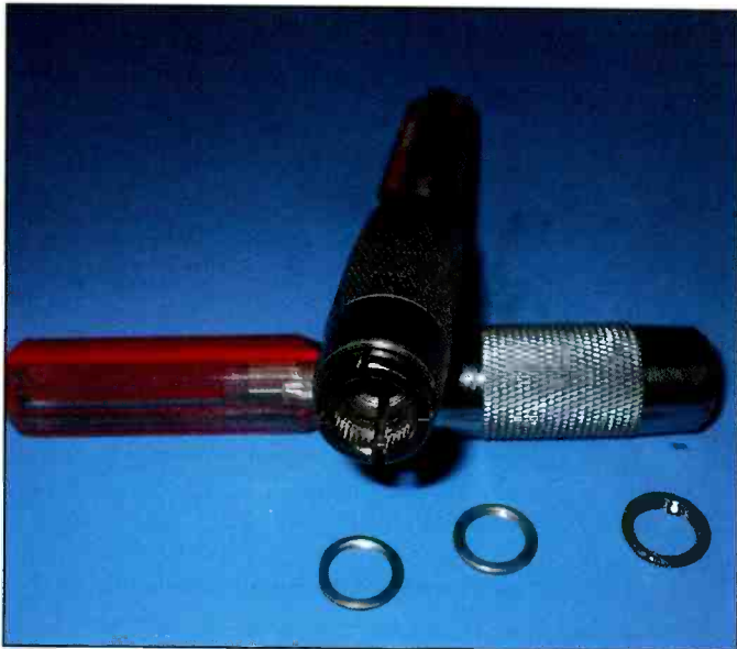
Photo C. Those decorative knurled finish nuts that are often seen on toggle switches require a special tool for removal or tightening. They are available from GC Electronics.
