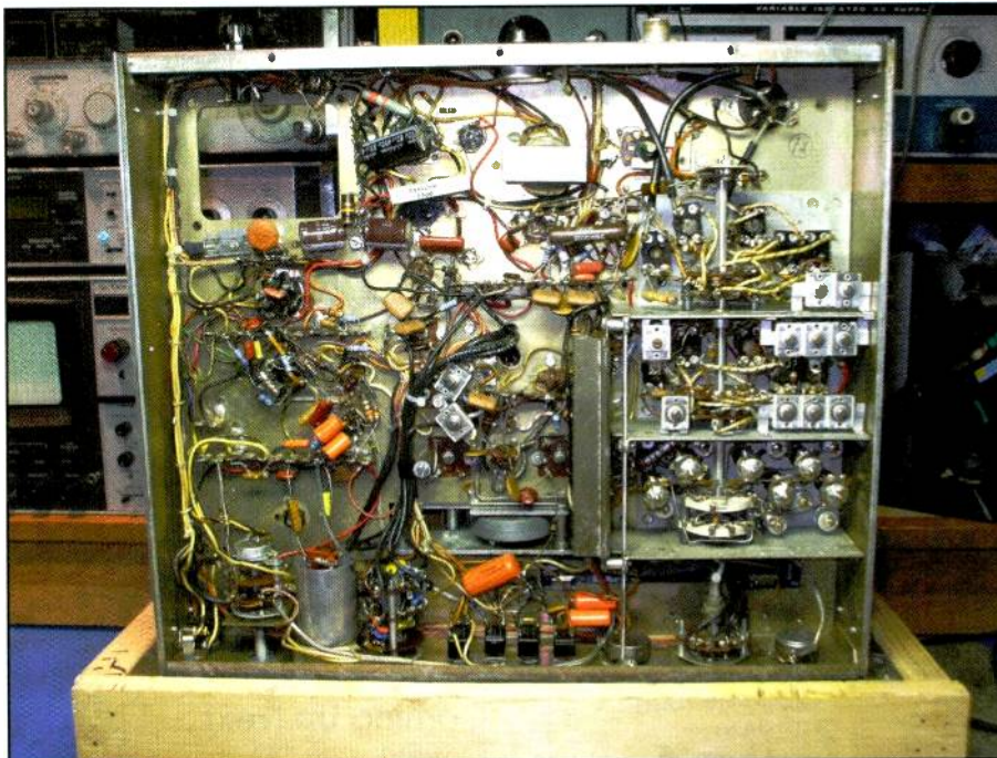
Photo H. The SX-101A chassis is heavy and requires support. Attempting to lay the radio upside down on a workbench can cause serious damage to tuning cores in several of the transformers.
