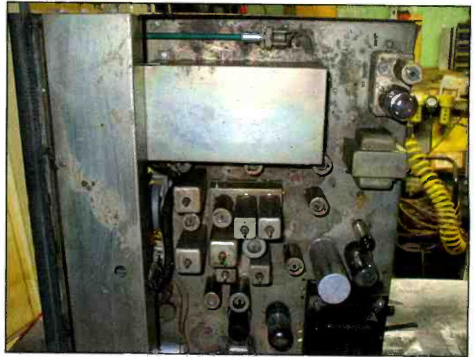
Photo E. Years of neglect took their toll, but the damage was less than we had to deal with in the HT-32 restoration. 409 cleaner applied vigorously with an old toothbrush removed most of the crud and corrosion.
