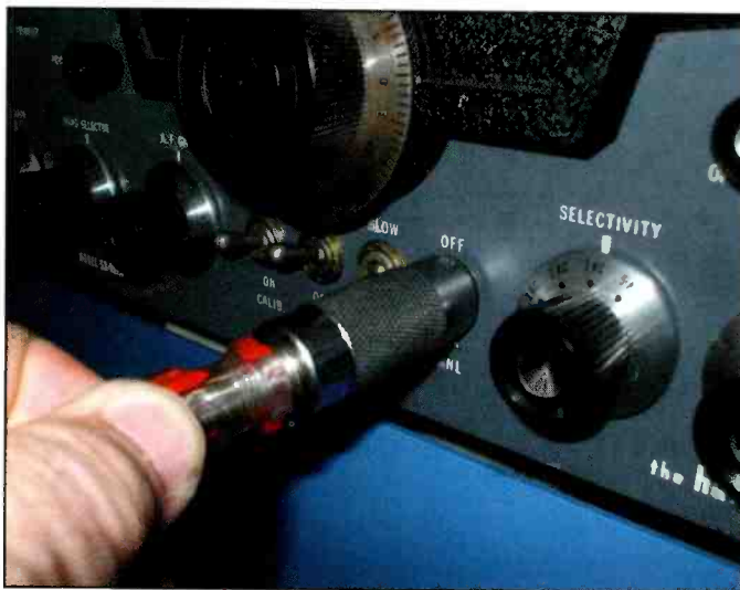
Photo D. Don't try to adjust the collet for the correct jaw size before engaging the tool. Instead, place the face of the knurled jaws over the knurled finish nut, and then tighten the collet until the jaws are firmly grasping the knurled nut surface.
