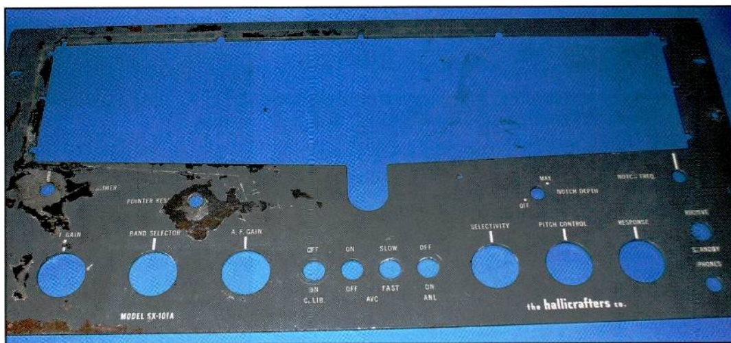
Photo A. The SX-101A was stored and forgotten in an attic for many decades before it was rescued. Paint was flaking from the front panel and there were areas of rust. A sad end for an old warhorse! (Photography by K1ZJH)
