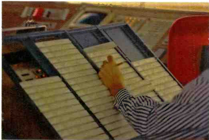
Remember Denver Stapleton Airport in Colorado? Here's a flight data position there before the facility moved to new digs in 1995. The controller is marking a flight progress strip that tracks the progress of aircraft flying in the area.
