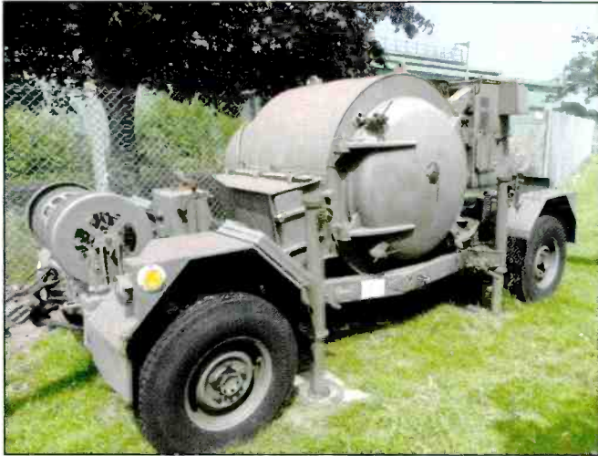
A mobile silent power unit was used to provide power for portable RADAR systems.
