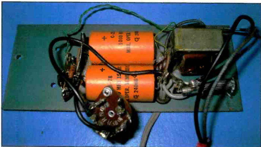
Photo F. The XP-2 AC power supply was an additional cost option for the Mohican receivers. The original supply is shown here.
