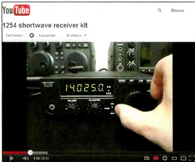
Photo C. The Ten-Tec Model 1254 is a general coverage communications receiver with a frequency range of 100 kHz to 30 MHz, powered by an included 15-VDC external power supply. "The best feature is that you build it yourself," writes WPC1CAT. To see a video of the 1254 in action, visit, < http://bit.ly/yzw43U >. (Internet screen grab)
