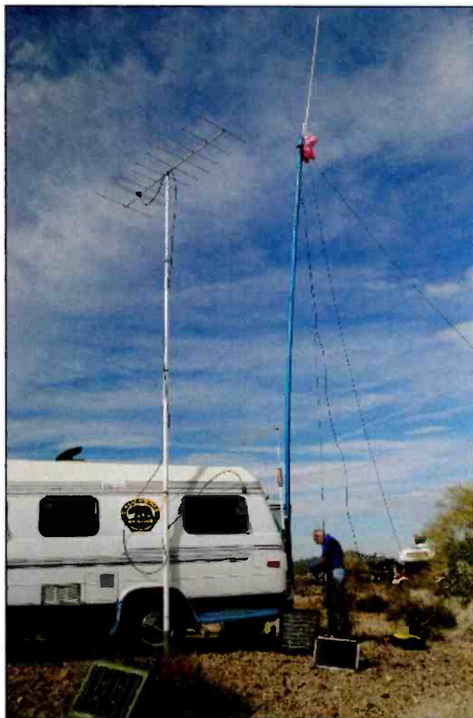
Photo A. Gordon West, WB6NOA, works 2-meter SSB DX via tropospheric ducting during a trip to the California desert. His van's wheel-mounted mast and compact Yagi combine to assure his VHF signal is getting out. (Images courtesy of WPC6NOA)
