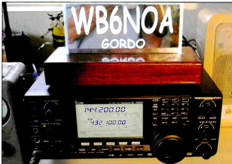
Photo B. Gordo's ICOM IC-9100 is tuned to 144.200- and 432.100-MHz upper single sideband (SSB) to assure he doesn't miss a minute of the tropo action.
