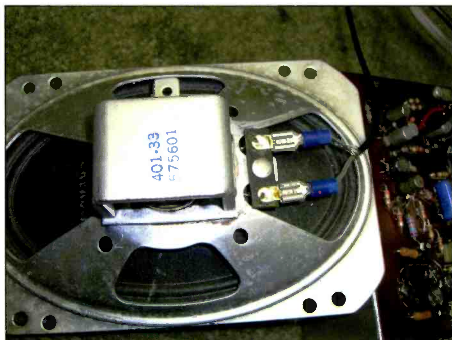
Photo I. Adding push-on female spade terminals for the speaker connections make it easier to remove and install the Mohican in its cabinet.
