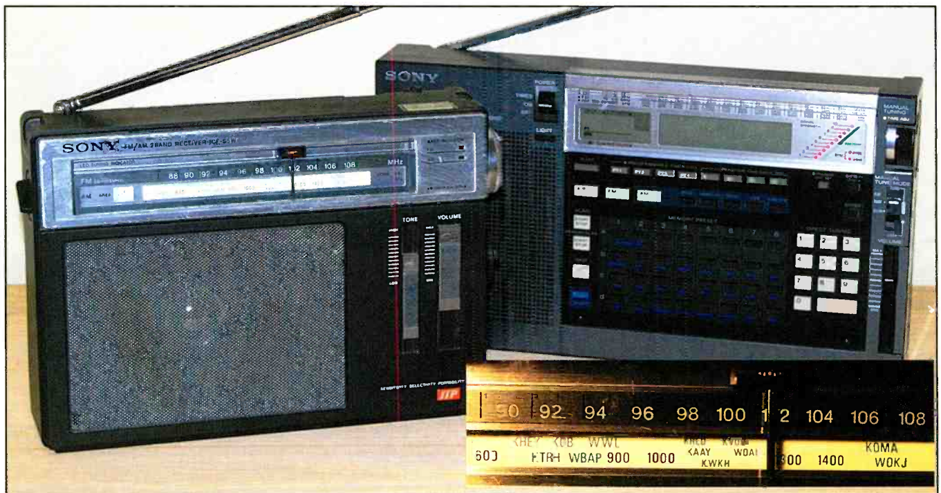
The Sony ICF-S5W and ICF-2010. Inset: Close-up of the S5W tuning dial.
