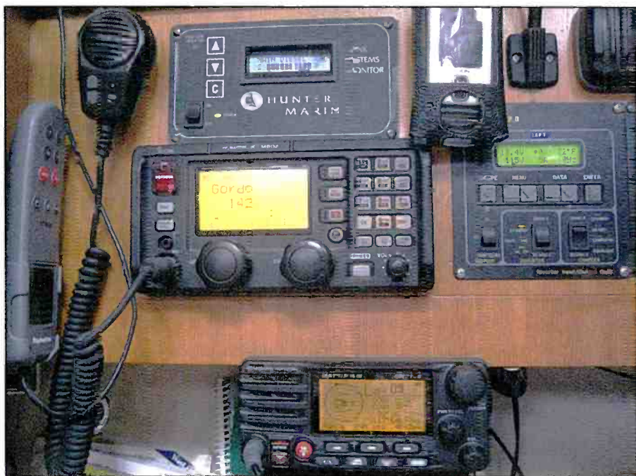
Here's a look at a typical sailboat DSC radio system.
