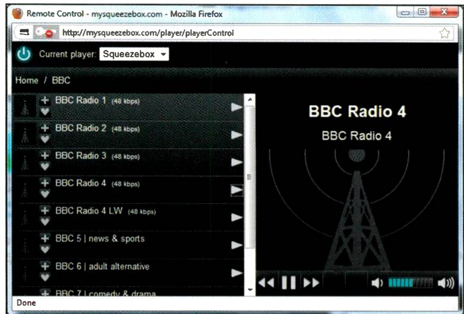
Figure 1. The Squeezebox Internet radio can be controlled over the Web through a Remote Control applet. Note the virtual power button at the upper left.
