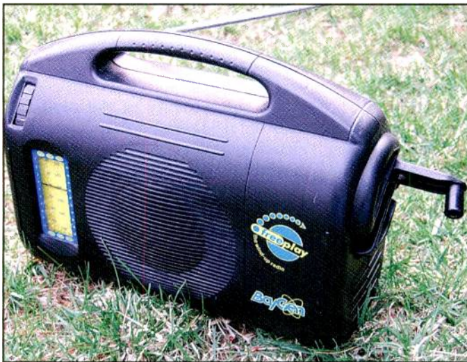
A wind-up clockwork spring powers the Baygen Freeplay.
