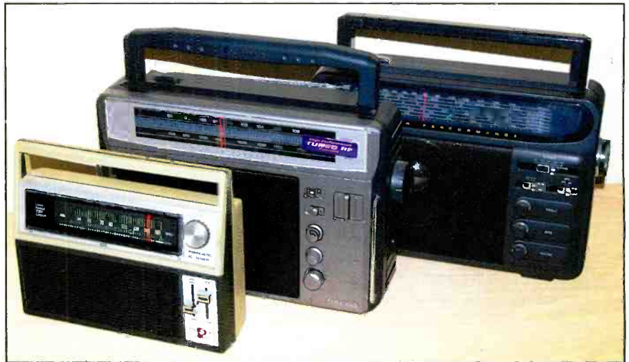
Tuned RF portables from Radio Shack: The Realistic TRF, Radio Shack 12-903, and Optimus — clone of a Superadio.
