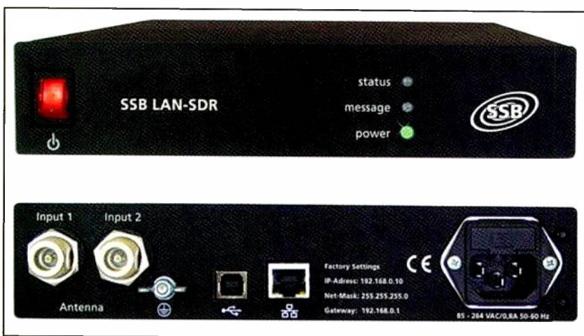
Figure 1. Front and rear shots of the SSB LAN-SDR. This is a most simple “black box” design with sophisticated capabilities built into the software. Note the use of ‘N’ connectors for the two antenna inputs.
