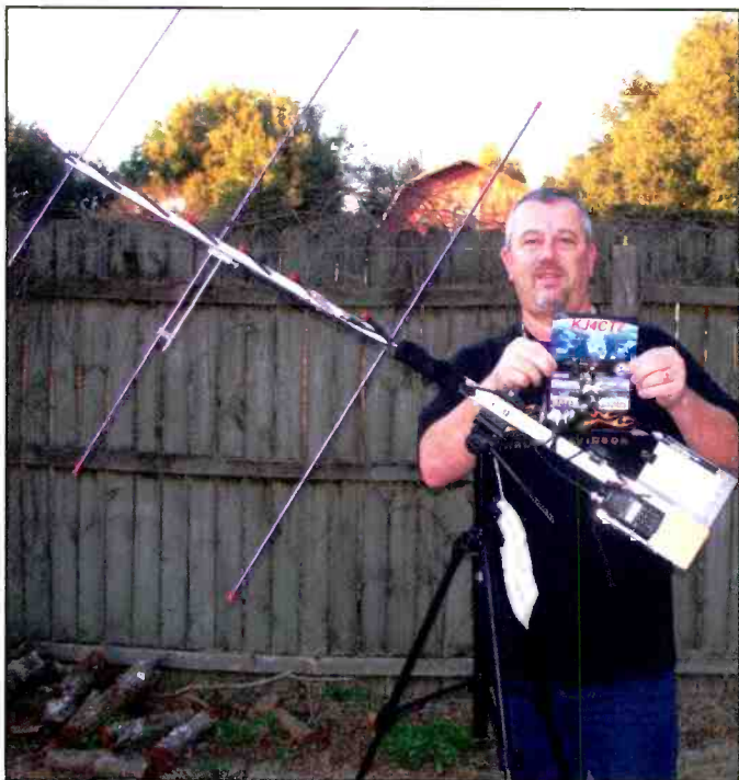
Ken Peakman, KJ4CTZ, of Florida, uses this setup to communicate with the International Space Station with his tiny Wouxun KG-UVD1P radio. The long boom antenna is aimed at the station. Note the radio mounted on the bottom end of the boom. Ken is showing off his QSL card and a QSL he received from the space station after talking to it with his Wouxun.
