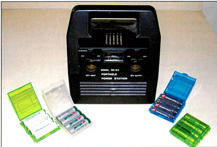
A selection of batteries, and a Portable Power Station, which contains a 7Ah gel-cell battery which will power a typical handheld scanner for at least 24 hours.
