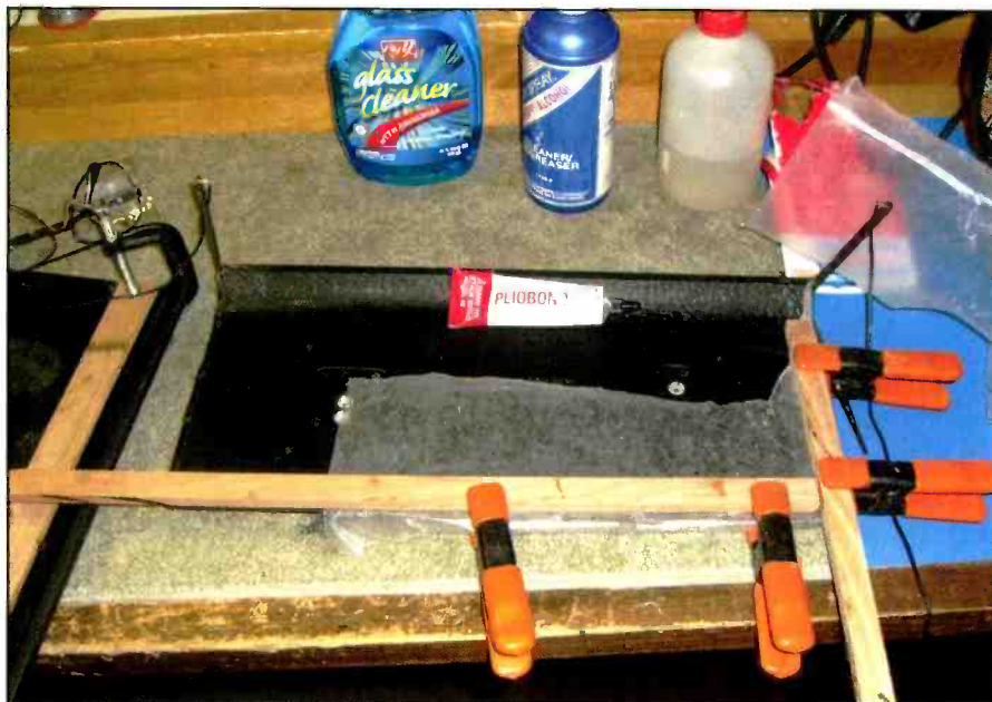
Photo D. Once re-glued, the seams should be held firmly against the cabinet using scraps of oak and wood clamps. Wax paper keeps the wood strips from being inadvertently glued to the cabinet!
