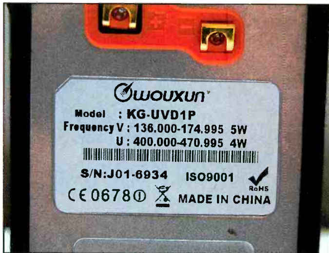
The inside of a UHF version of the Wouxun KG-UVD1P shows its frequency coverage of 136–175 and 400–471 MHz, and shows the power output as 5 watts on VHF and 4 watts on UHF. (Photo by Chuck Gysi, N2DUP/scancomm.net)
