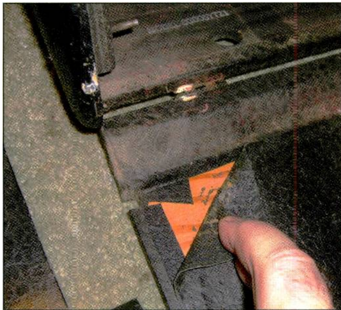
Photo C. Years of storage and changing seasons can cause the old glues to dry out and weaken, resulting in loose sections of stag material, especially at the edges and seams. Note the wire leads that are attached to the hinge arms. These wires connect the WaveMagnet antenna to the radio. The wires and hinge pivot points are hidden beneath the top plate section when the radio is assembled.
