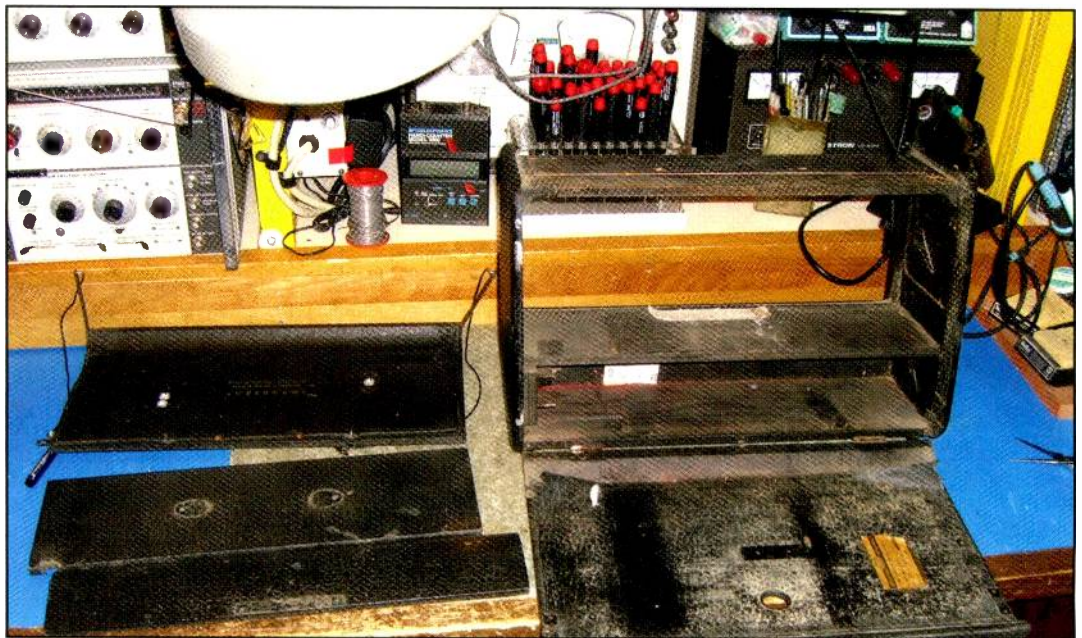
Photo A. The Zenith Trans-Oceanic cabinet has been disassembled into five sections. The largest is the main cabinet. At left, going from top to bottom, is the top front lid, top plate, and the small door for the instruction booklet located in the lower front section of the radio. The rear cover is just below the main cabinet box.
