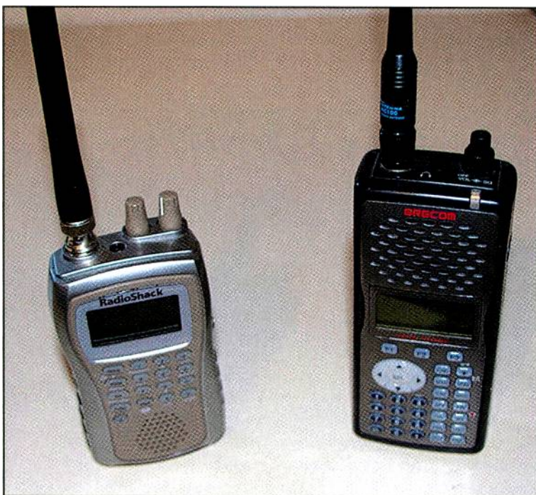
Two handy scanners for aviation monitoring. On the left is a Pro-83 scanner for monitoring civilian air frequencies; on the right is a PSR500 monitoring the UHF military frequencies.
