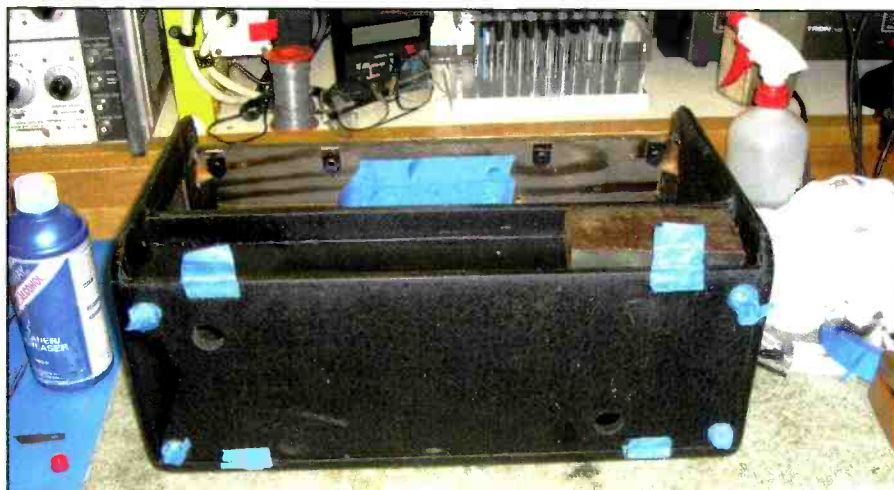
Photo E. It's a good idea to remove any pieces (metal feet, hinges, etc.) that shouldn't be painted. If they aren't removed, they should be covered with masking tape.
