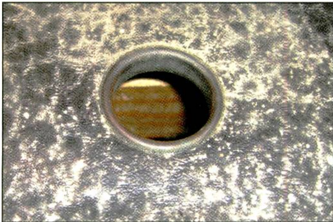
Photo B. White mold is commonly seen on the stag covered Trans-Oceanic radios. The glues and materials provide a fertile growing medium for the mold. Luckily, it's easily removed with a damp rag and soap.
