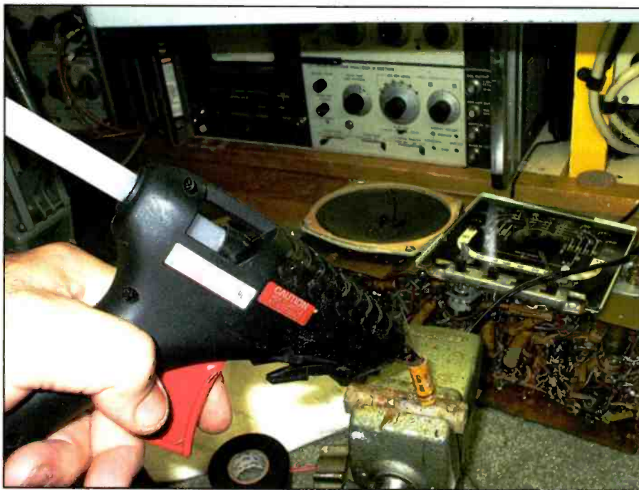
Photo J. This shows a hot glue gun being used to fill the voids around the replacement Mylar cap, which will be hidden inside the old Zenith brand-name cardboard shell. Use a capacitor with a modern equivalent of close value and with a voltage rating that is equal to or higher than the original.
