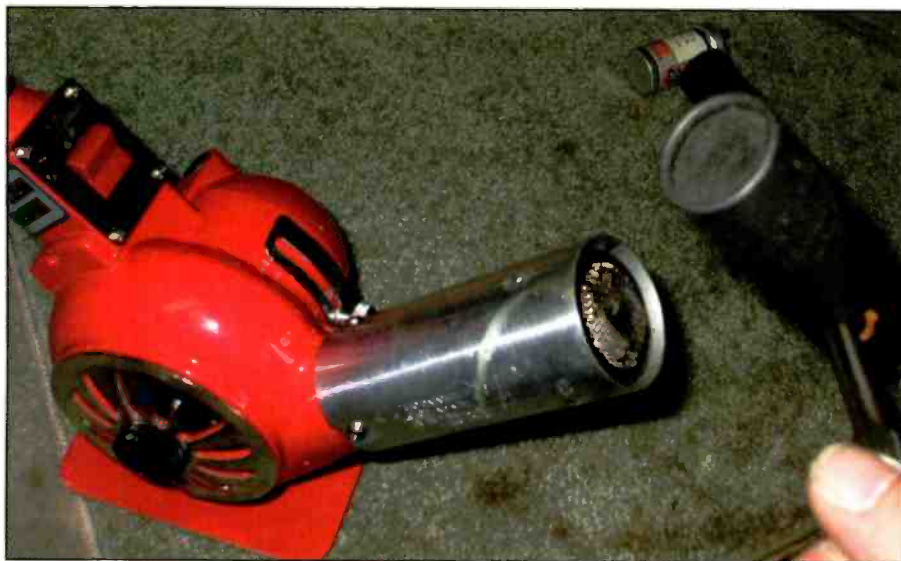
Photo H. Although this photo shows a hot air gun being used to heat one of the set's two electrolytic capacitors, the procedure is similar for heating a removed waxed paper capacitor. There are safety-related concerns that must be observed when heating electrolytic caps that will be discussed in a later column.
