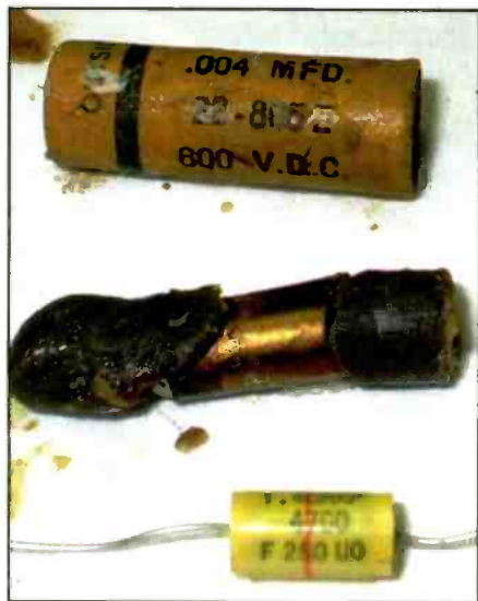
Photo I. By gently and evenly heating all sides of the tubular wax capacitor's outer cardboard shell, the wax used to seal the capacitor will soften and permit removing the innards (photo center), leaving the hollow shell (photo top) to be rebuilt with a modern axial lead Mylar capacitor (bottom) hidden inside.
