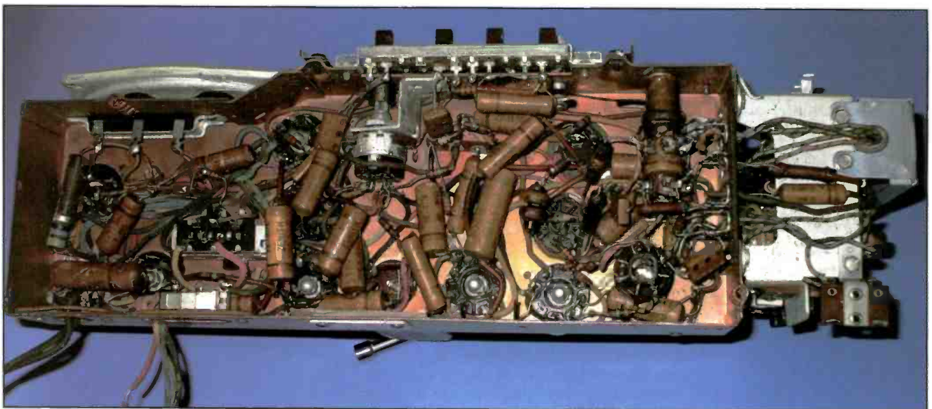
Photo F. The Zenith 8G005 is one of the most complex of all the Zenith tube Trans-Oceanic models. It is the only tube model featuring a push-pull audio section. As can be seen under chassis, the components are densely packed. This is not a good set for beginners or intermediate hobbyists to attempt restoring.
