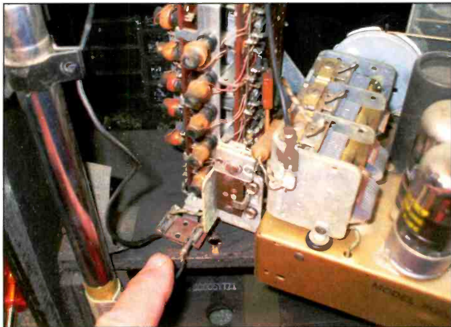
Photo D. Before removing the chassis, these three antenna leads should be unplugged and moved clear. Two are for the AM loop antenna mounted on the top cover, and the third is for the shortwave whip antenna mounted at the far right. Be very careful not to damage the delicate coils on the band-switching coil tower assembly.
