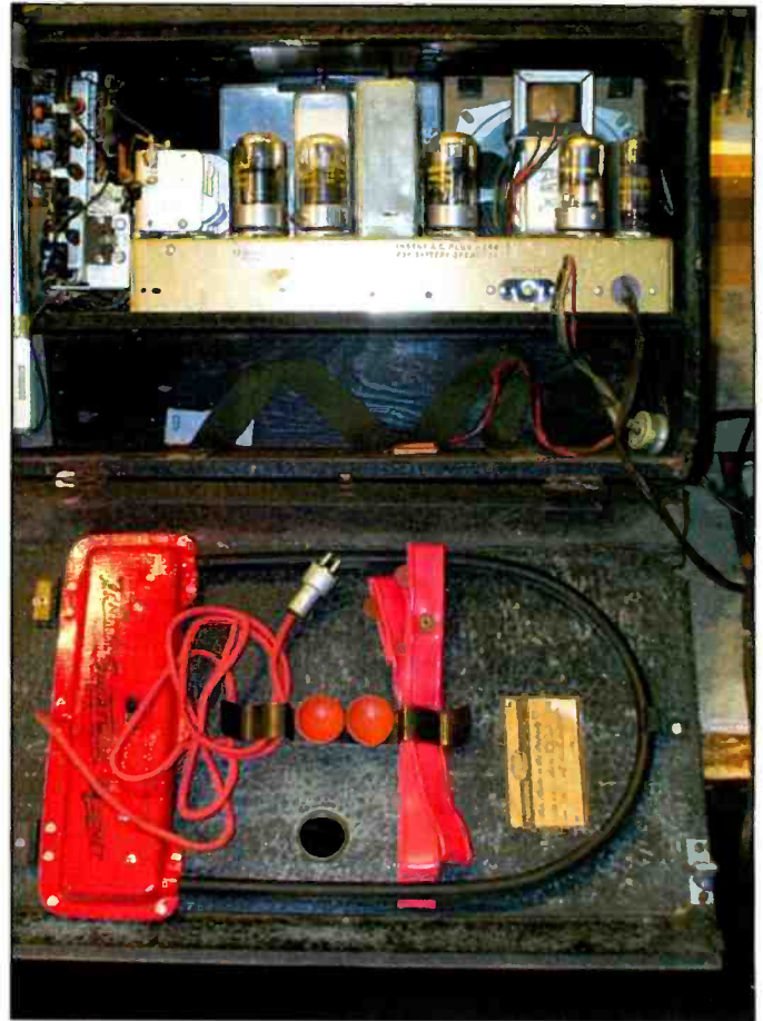
Photo C. For this photo the rear cabinet door is opened to show the radio chassis, battery compartment below, and the various antenna accessories that are stored attached to the rear cover. Look at all those tubes! This is an eight-tube chassis—the highest tube count of all the Zenith Trans-Oceanics! Missing accessories, or damage to the stag fabric, will greatly diminish the value of the set.
