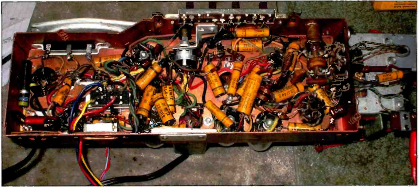
Photo G. I'm jumping ahead a bit in our story line, but I wanted to show how I feel a restoration should be done for sets of this caliber. I took extra steps and time to preserve the under chassis appearance, in part because this set used Zenith brand-name marked parts. Again, this is a personal choice. Some restorers don't worry about what can't be seen under chassis; others will feel I didn't go far enough.
