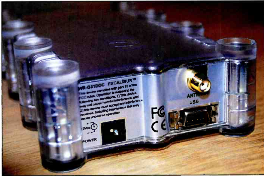
Here's a close-up view of the Excalibur rear panel connections for 12-VDC power, USB, and antenna.
