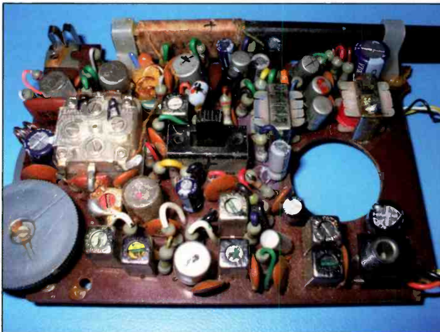
Photo A. As we first saw in October, the top view of the Jetstream printed circuit board shows the radio's extremely tight component density.
