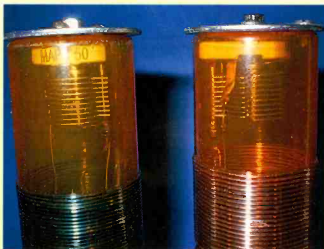
Photo E. This close-up shows how Bob has mounted two screwdriver-type APC-style air trimmer capacitors in his coil forms. The capacitor bodies are kept well out of the actual coil winding area on the form; this preserves the coil Q factor.
