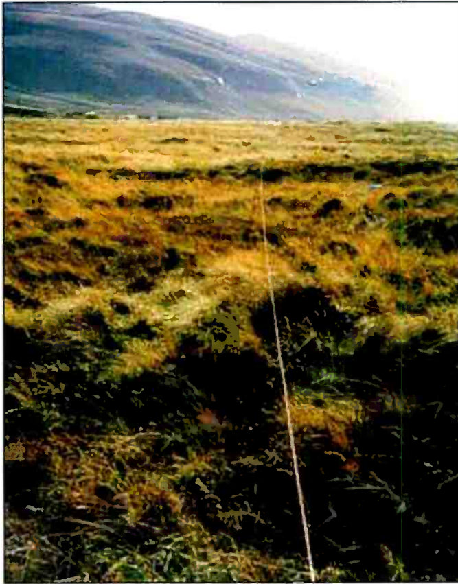
One of the Beverage antennas extends across the sheep grazing fields of Sheigra.
