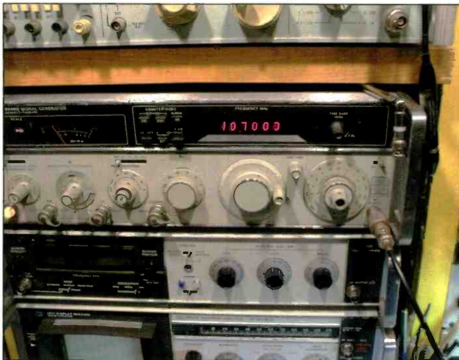
While almost any available signal generator would do for the IF and BCB alignment, I used one of my shop's HP-8640 lab-grade generators for this procedure. Note that in this photo the generator was locked to 10.7 MHz for aligning the aircraft band's 10.7-MHz IF stages.
