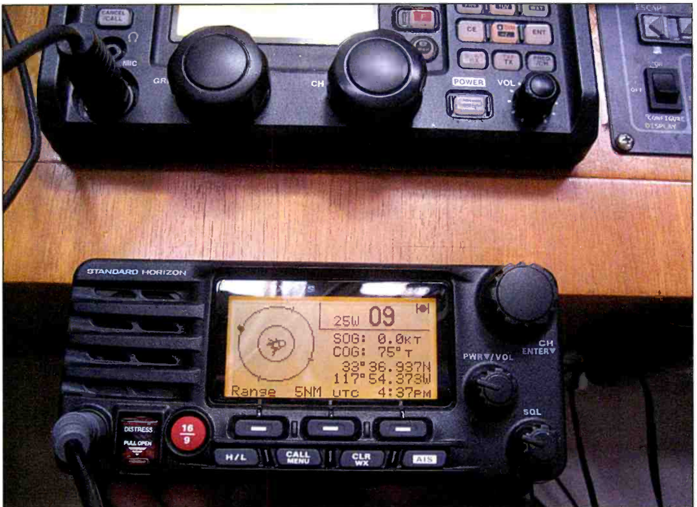
The shore station license may grant both SSB (top) operation as well as VHF operation on land (bottom radio, tuned in to automatic position finding).
