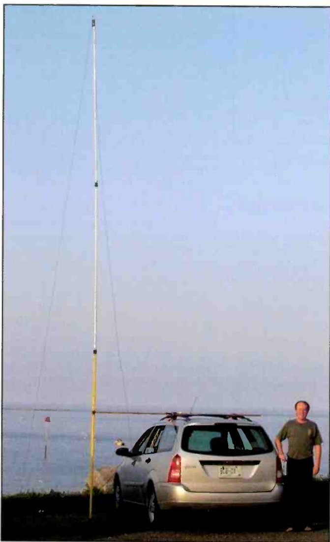
"Broadcast Technology" columnist Bruce Conti stands by his Delta antenna supported by a 23-foot collapsible painter's pole.
