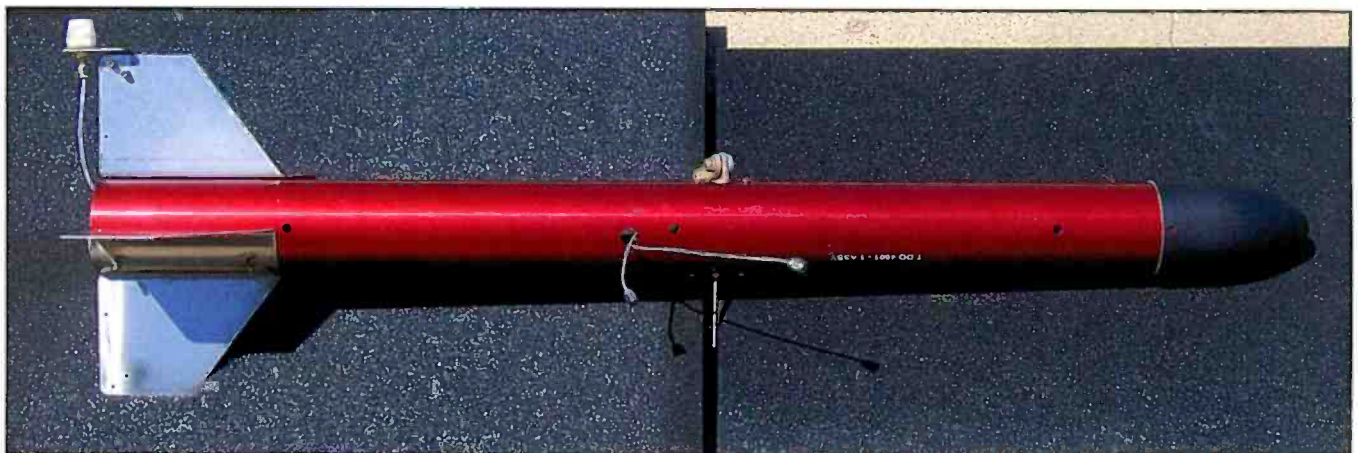
Photo A. Decoy for Monopulse seekers.
