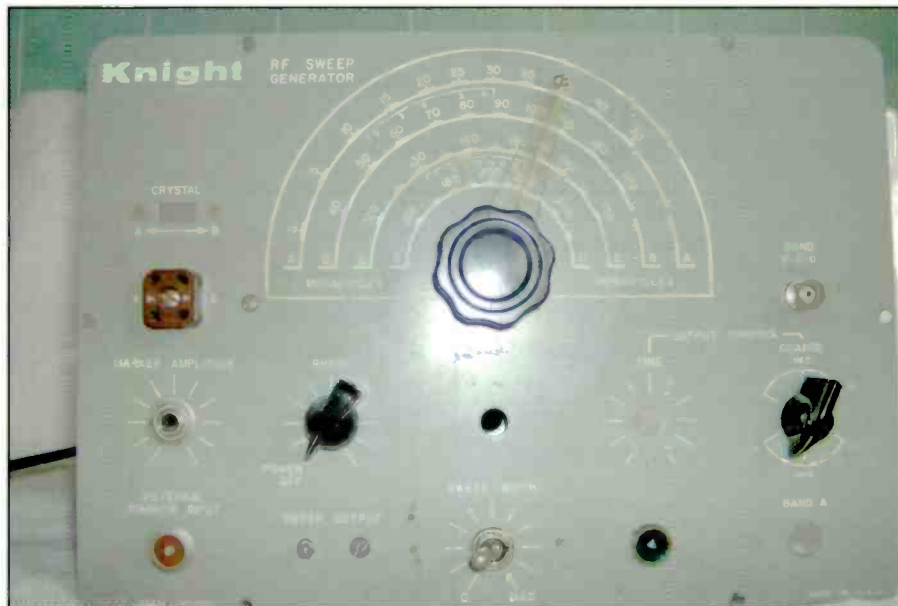
Photo A. Here's another one of Richard's Night Hawk efforts. Like the receiver shown last time, it is housed in a defunct test equipment enclosure. This set uses the One-Tube All-Bander plug-in coil set.
