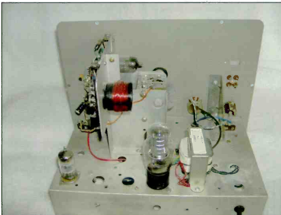
Photo B. An inside peak at what's lurking behind the dials. Note how Richard was able to make good use of many of the original components, such as the power supply, in this version of the Twin-Tube Night Hawk receiver.
