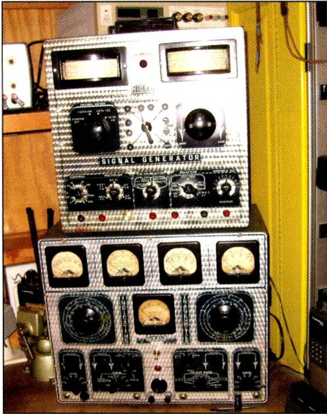
Photo A. Thanks to Alan Douglas, I am now the proud owner of this handsome 188X signal generator. It's shown with my Hickok Indicating Traceometer, another gorgeous vintage instrument sporting a machine finish front panel!
