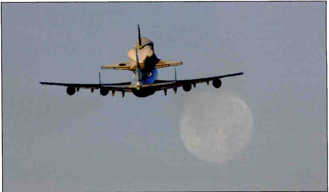
Photo C. Space Shuttle Atlantis during a 2007 piggyback ride on a modified Boeing 747. (NASA photo by Carla Thomas)
