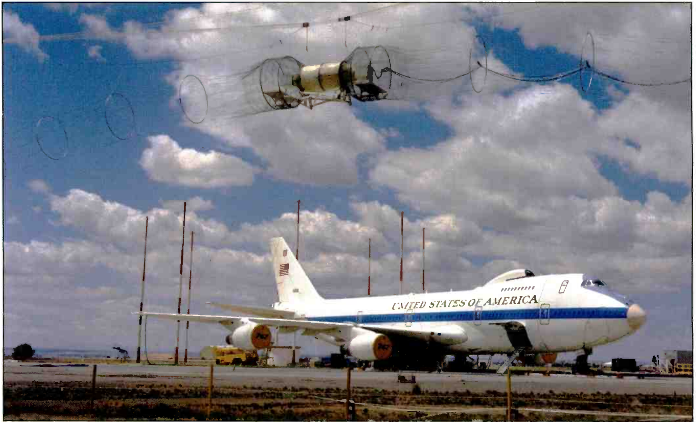
Photo B. An E-4 advanced airborne command post (AABNCP) aircraft being tested on the EMP simulator at Kirtland AFB, New Mexico. (USAF photo)
