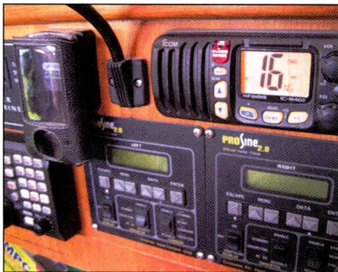
Channel 16, the International Distress frequency, must be monitored any time a marine radio is on and the vessel is underway.
