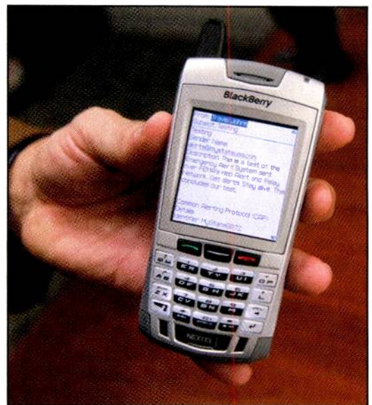
Photo A. An Internet-based textual test alert displayed on a wireless telephone device. (Courtesy Sandia National Laboratories)
