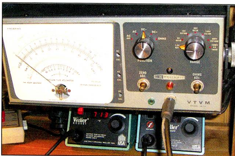
Photo A. The IM-13’s gimble bracket allows mounting under a shelf or on top of the workbench. The plastic meter cover has been removed to reduce glare in the photographs.
