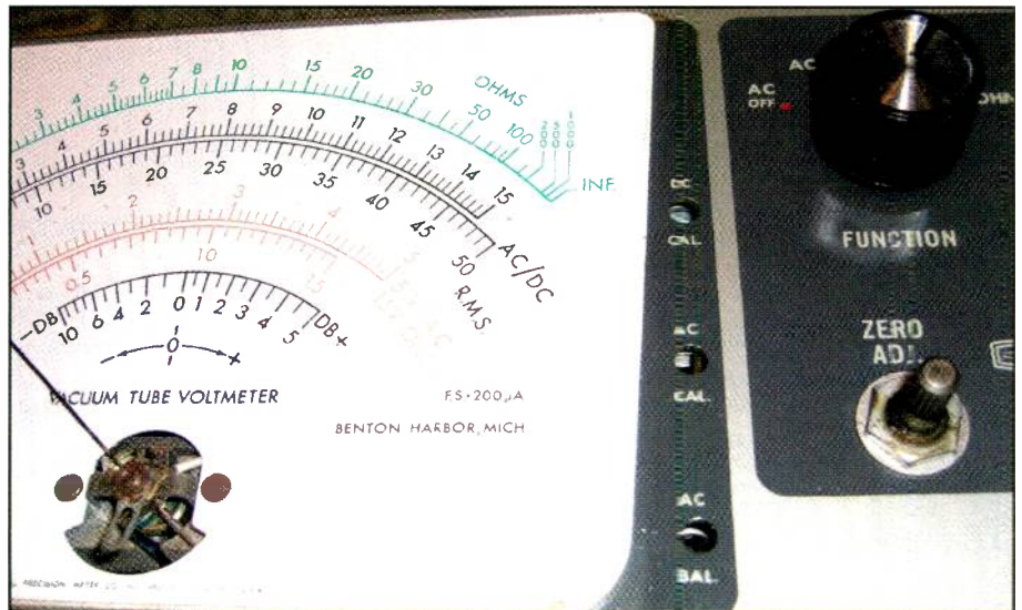
Photo B. Three holes to the right of the meter body provide access to the AC balance, AC calibrate, and DC calibrate trimmers. Just to the left of the 1.5-vDC meter scale you'll see a small red dot. That's used for the DC calibration when a fresh carbon zinc battery supplies the calibration voltage.
