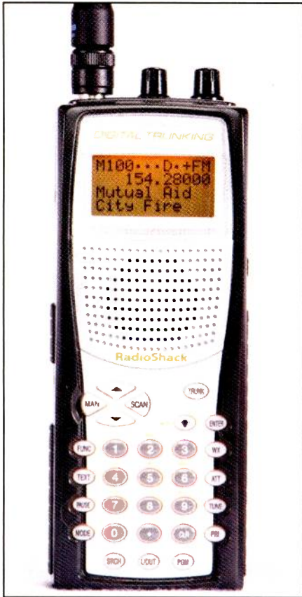
This RadioShack model is a full-fledged trunktracking scanner with lots of bells and whistles in a handheld package. Note the Alpha Tags displayed for Mutual Aid (Channel) and City Fire (bank).
