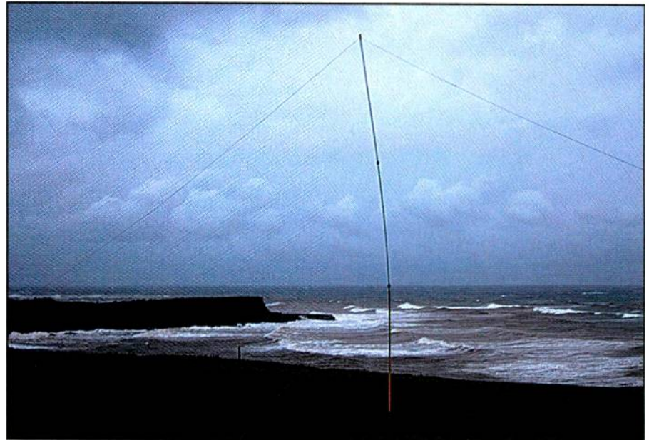
The Delta terminated loop antenna takes a beating during stormy weather.
