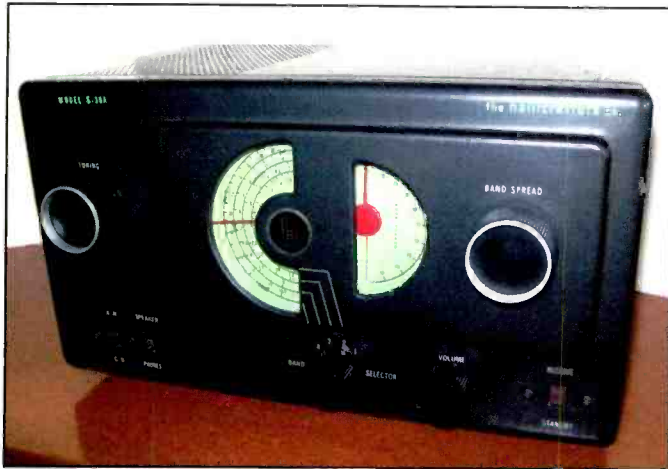
Photo D. The S-38A used a five-tube lineup, and the adjustable front-panel CW Pitch control was eliminated. These moves probably saved Hallicrafters a considerable amount of money, but the savings probably weren't passed on to the consumers! (Photo courtesy Ed Engelken)
