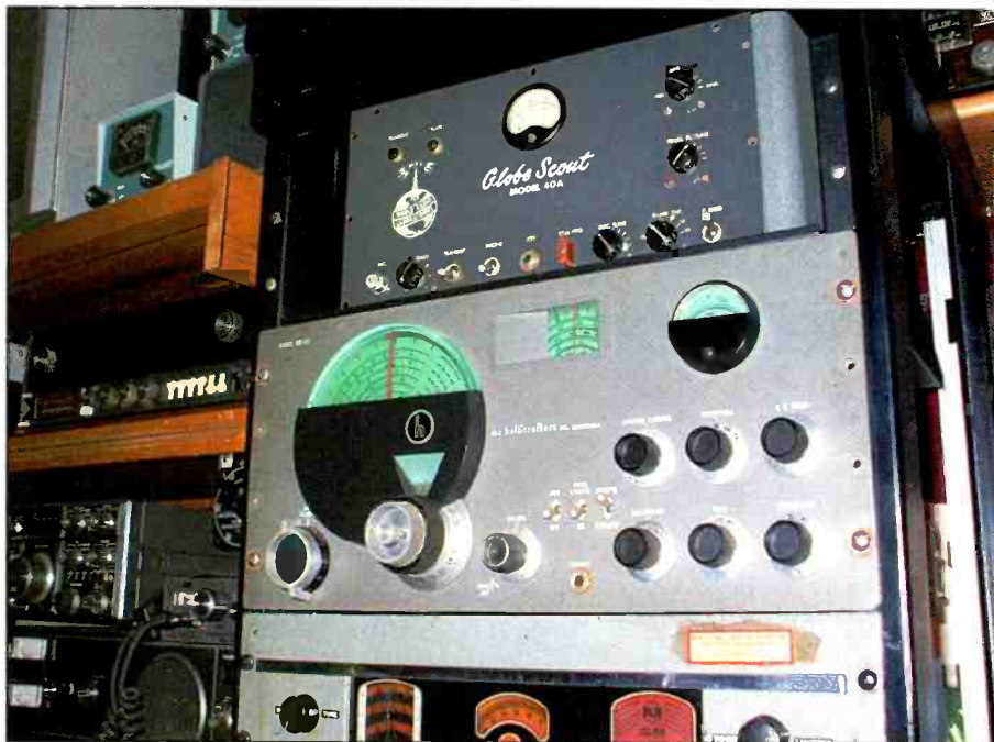
Photo A. The machine-age styling of the SX-42 receiver was the work of famed industrial designer, Raymond Loewy. The receiver is rack-mounted in the author's radio shop. The unit mounted below that, and partially visible, is an RCA model AR-88 World War II receiver.
