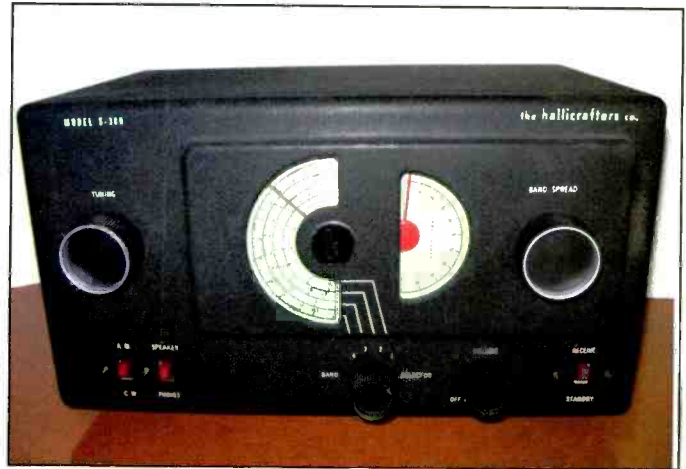
Photo E. To meet more stringent UL safety requirements, the S-38B introduced needed improvements to reduce shock hazards on these AC/DC powered hot-chassis sets. Many of the control shafts were changed to a non-conducting material to further reduce the chance of exposure to raw AC line voltages if a knob were removed. (Photo courtesy Ed Engelken)
