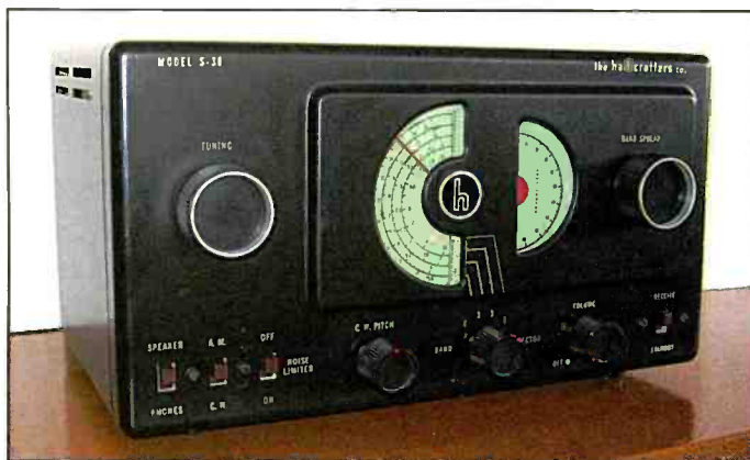
Photo B. The S-38 receiver was at first produced with a flat black finish. Note the presence of the BFO Pitch control, which is missing on the S-38A and later models. The early S-38 employed a six-tube lineup. (Photo courtesy Ed Engelken)
