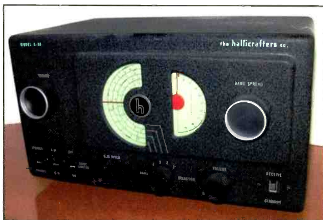
Photo C. This S-38 has a black-wrinkle finish, indicating that it comes from a later production run. (Photo courtesy Ed Engelken)
