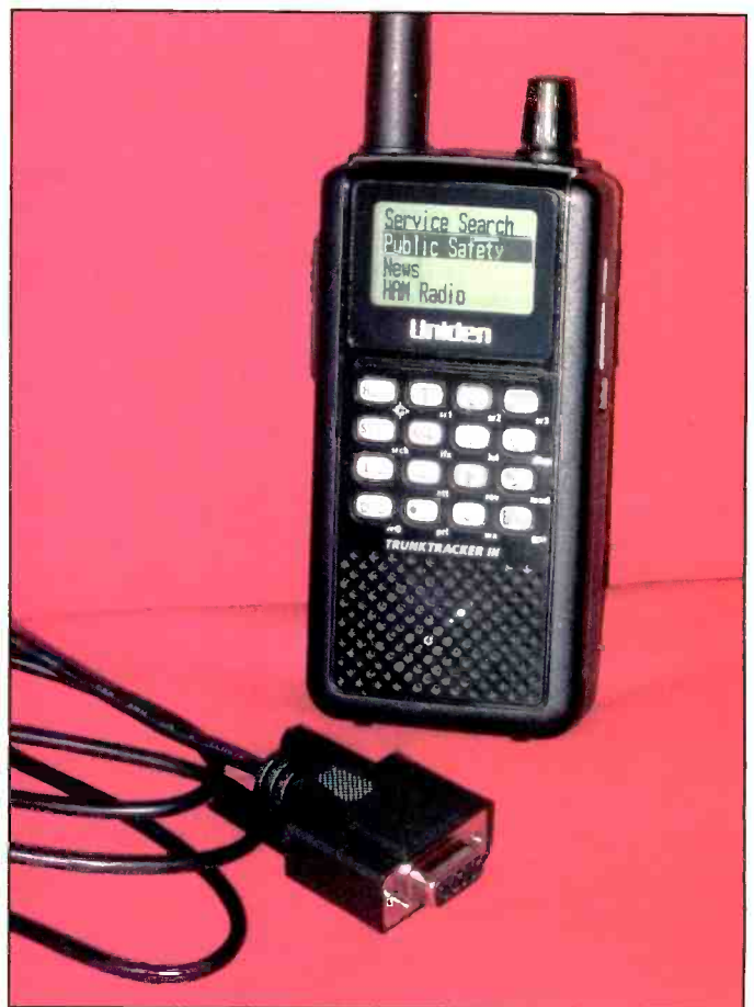
PC Control/Programming allows you the option of remotely programming and controlling the BC346XT scanner.
