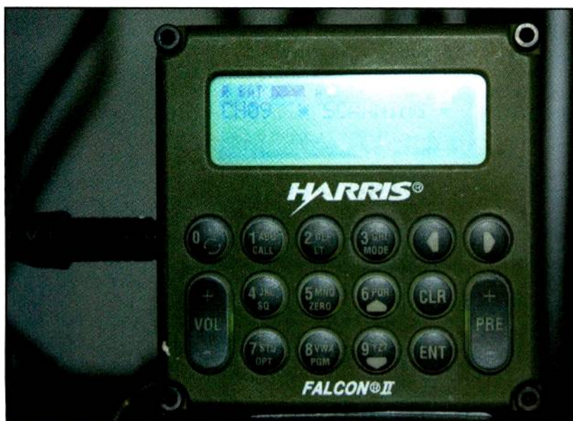
Like Codan, Harris Radio also utilizes ALE (see text). This radio is scanning channels waiting for an incoming message.
