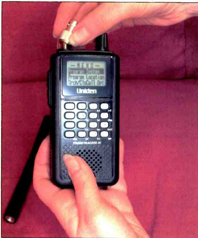
The Uniden BC346XT allows for both SMA and BNC antenna connections, providing plenty of flexibility in scanning.
