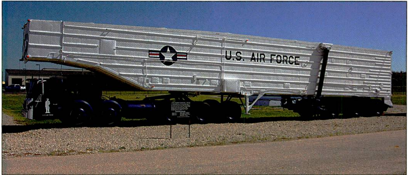
A Boeing Minuteman Transporter-Erector, used by the 351st Strategic Missile Wing to ferry missile boosters to and from missile silos. It was retired in 1993 to static display at Whiteman AFB. (U.S. DefenseLink photo)
