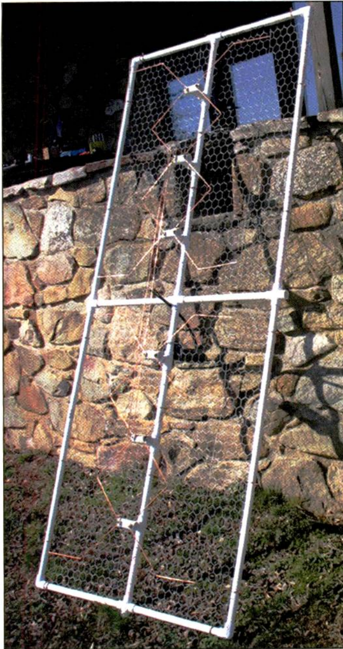
Photo B. This two-bay Gray-Hoverman array with screen reflector may get your neighbors talking, but its 15- to 18-dB gain for UHF TV—with tremendous front-to-back and beamwidth performance—will make you a TV DX champion. These antennas, generously released to the public under the GPL open-source license, can be designed for single frequencies. I wonder if anyone's used them for ham or scanner applications? For more info see www.digitalhome.ca .
