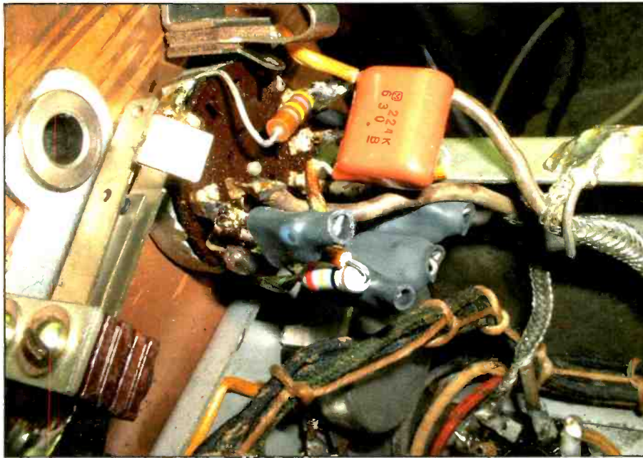
Photo B. A view of the replacement resistors used to rebuild the AF volts channel attenuator. Black heat shrink tubing kept things neat whenever two or more resistors were used to replace a single odd value. The attenuators for the AF and DC channels both use resistors and are very similar in appearance.
