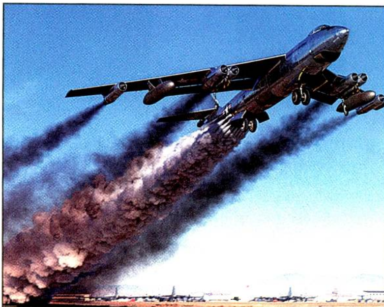
A B-47B using rocket assisted take-off on April 15, 1954. (Public domain photo)
