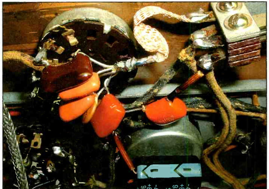
Photo C. This is a close-up of the capacitors used in rebuilding the oscillator channel attenuator.
