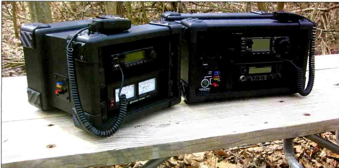
Mark Mantia, WN8ATM, has been one busy guy. In addition to designing, fabricating, and marketing a special stand for the venerable Yaesu FT-817 multi-mode transceiver (see text), he also found time to develop and fabricate some really nice-looking and extremely functional EmComm BOBs that will help the ARES/RACES EmComm volunteer better function as an emergency communicator.
