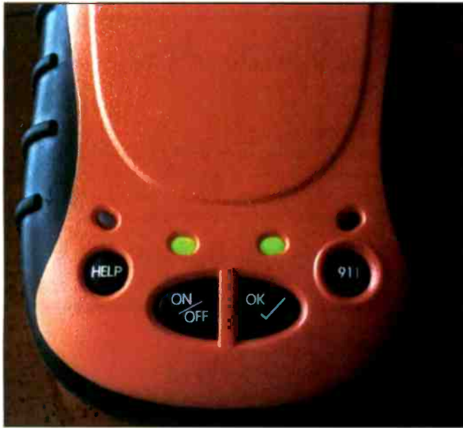
SPOT's LEDs indicate the status of GPS reception, outgoing messages, and activation of the help or 911 key.
