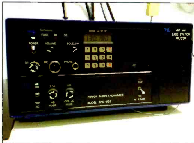
An ARINC ground station radio; this one happens to be owned by US Airways. (Photos by the author)
