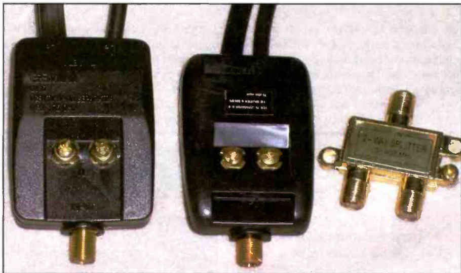
Photo E. FM band splitters to take the FM signal off an outdoor TV antenna.
