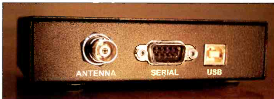
The SDR-IQ rear panel with antenna, serial, and USB connectors.
