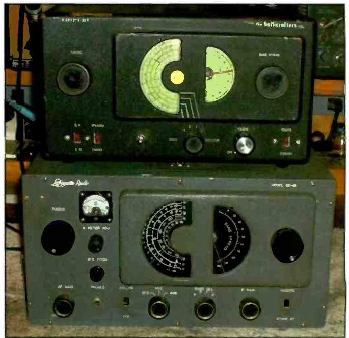
Photo A. Placing a Hallicrafters S-38 atop the later Lafayette HE-10 is a good way to show the obvious outward physical similarities between the two receivers. Despite the similarity, the HE-10 was far more advanced: it featured a transformer power supply, an S-Meter, a tuned RF stage, and two IF stages. The partially assembled KT-200 kit cost $64.50.
