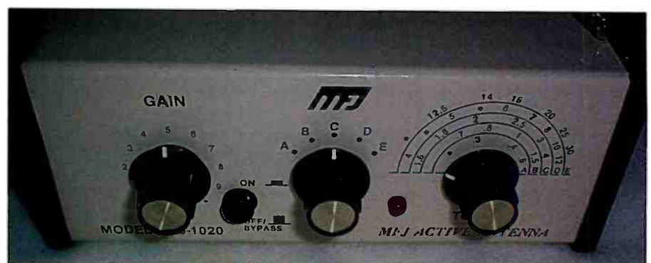
Photo B. The MFJ-1020 HF active antenna with preselector.
