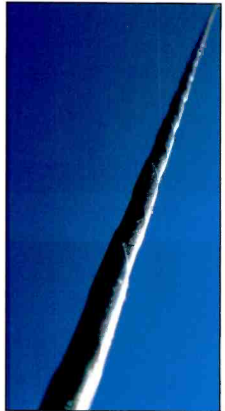
Photo G. Antenna flutes put an end to singing in the wind, if not in the rain.
