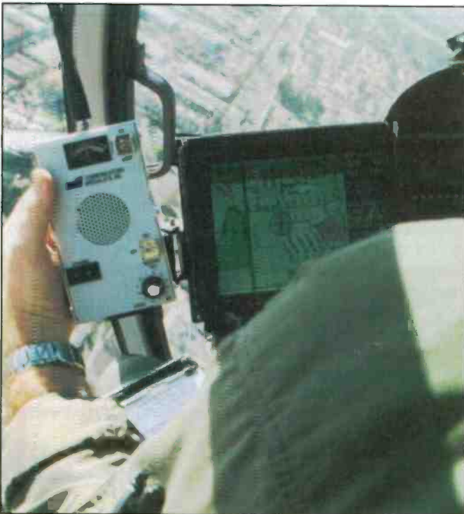
Going the distance—helicopter long-range radio trials on the ← 222-MHz band proved the usefulness of these locator tags.
