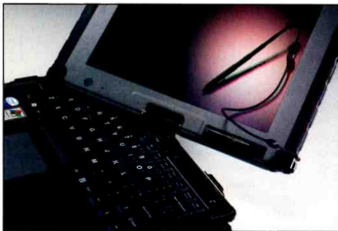
The GETAC V100 notebook offers a 120 GB shock-mounted removable hard drive, integrated bluetooth, and wireless networking capabilities in a water-resistant, rugged magnesium alloy case and is ready for mounting in any emergency vehicle.
