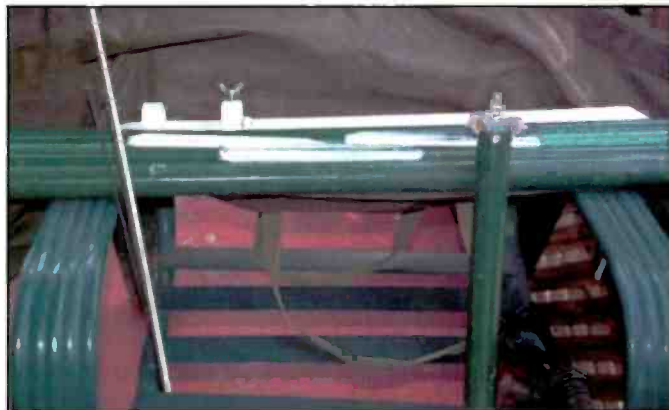
This is a shot of the portable mast system from Fair Radio Sales. This configuration offers a very light 20-foot fiberglass mast with 2-meter ground plane antenna and coaxial cable.
