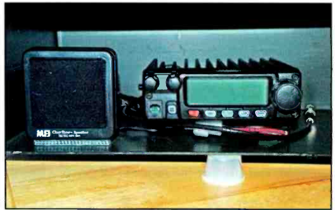
Trial fit of the FT-2800 2-meter FM radio set with the MFJ speaker in the 40mm ammo can.
