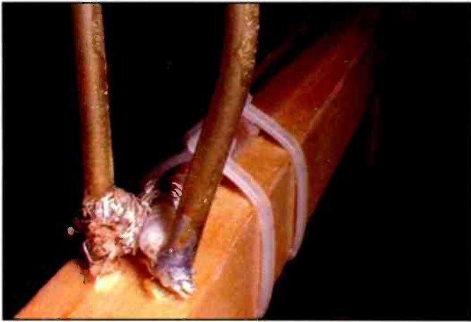
Photo E. Attaching the coax to the driven element.
