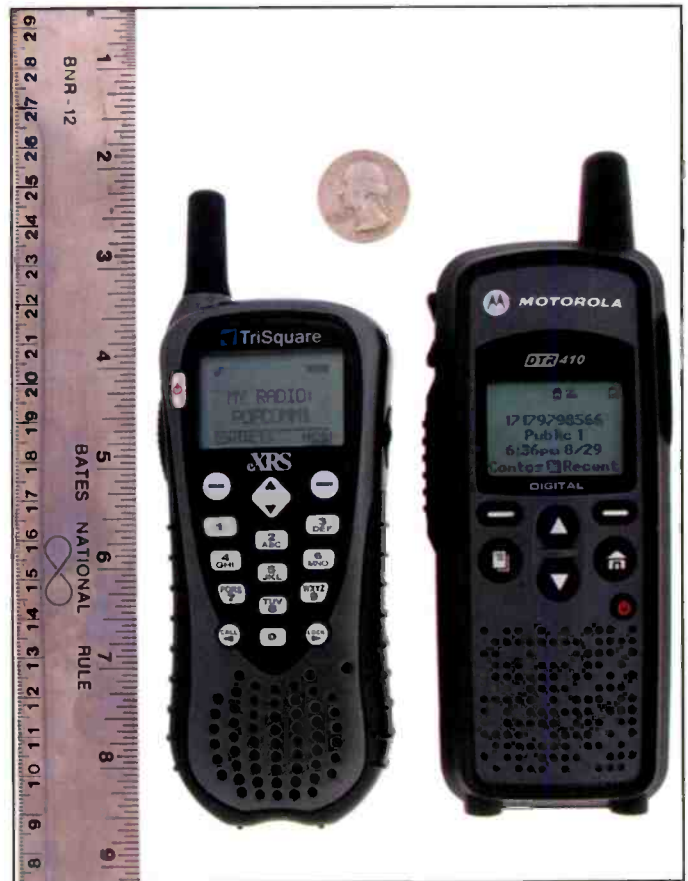
TriSquare’s TSX-300 and Motorola’s DTR-410 FHSS radios—the dynamic duo of the digital domain! Now the general public can get in on the FHSS radio action.
