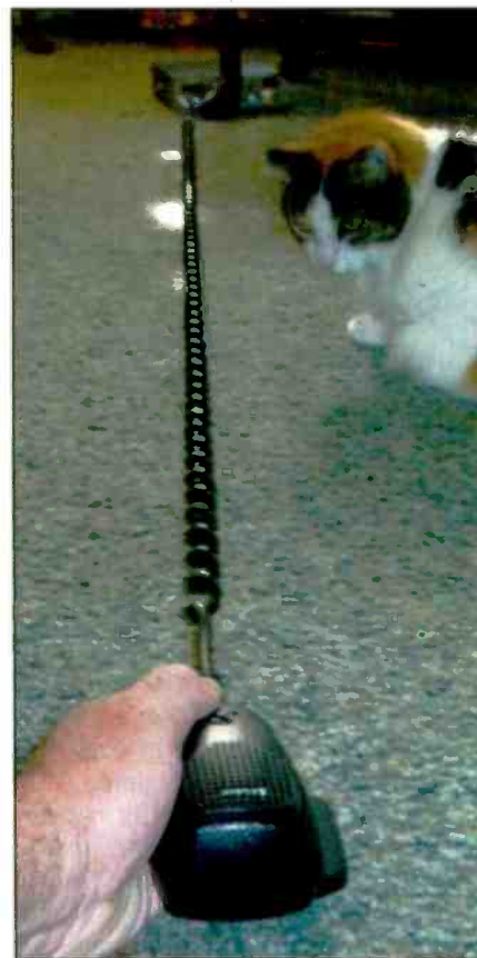
Here's the mic cord stretched to the limit of about six feet. The radio was propped against a chair leg for our quick test (don't do this to your mic cord!).
