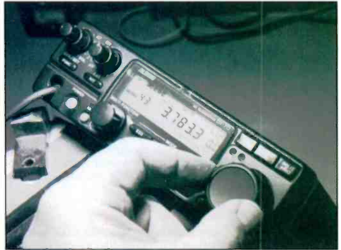
The Alinco DX-70 with its remote head. It uses a large remote cable for the connection between the radio's main body and head. (Photo by Bill Alber, WA6CAX)
