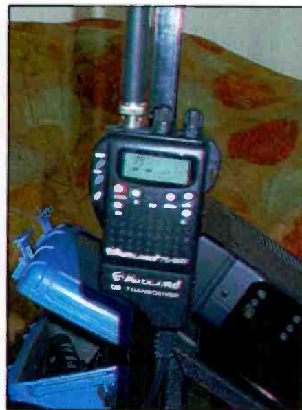
The Midland 75-822, shown here monitoring Channel 19, is a perfect fit! It's a full-power 40-channel handheld (and mobile) CB that once again demonstrates its versatility for all kinds of communications needs and fun.
