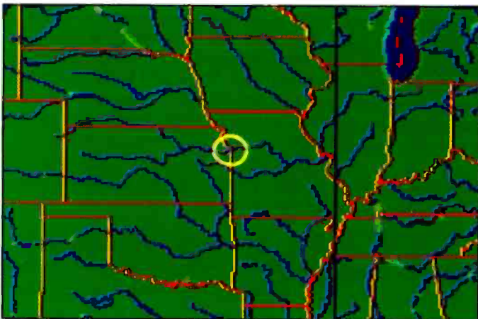
Figure 1. Typical line-of-sight circle of a VHF signal from a 1,000-foot tower in Kansas City.
