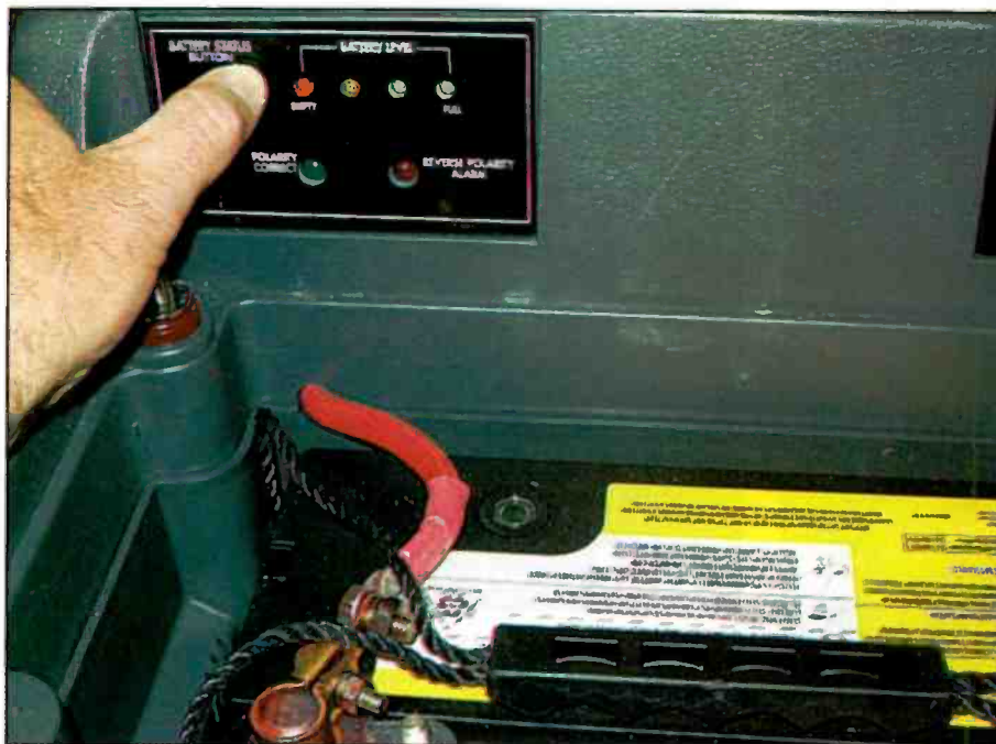
The status lights on the ElectroMate show a full battery charge, but as with all other power units, always take an independent voltage reading.
