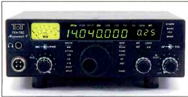
Ten-Tec's Argonaut V has the benefits and features of IF-DSP in a modern 20-watt HF all mode transceiver. Power is adjustable from 1-20 watts output. (Photo courtesy Ten-Tec).
