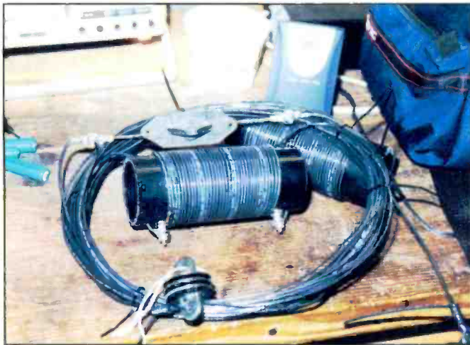
A simple dual-band dipole can be constructed for under $20. (Photo by Don Wilson, N9ZGE)
