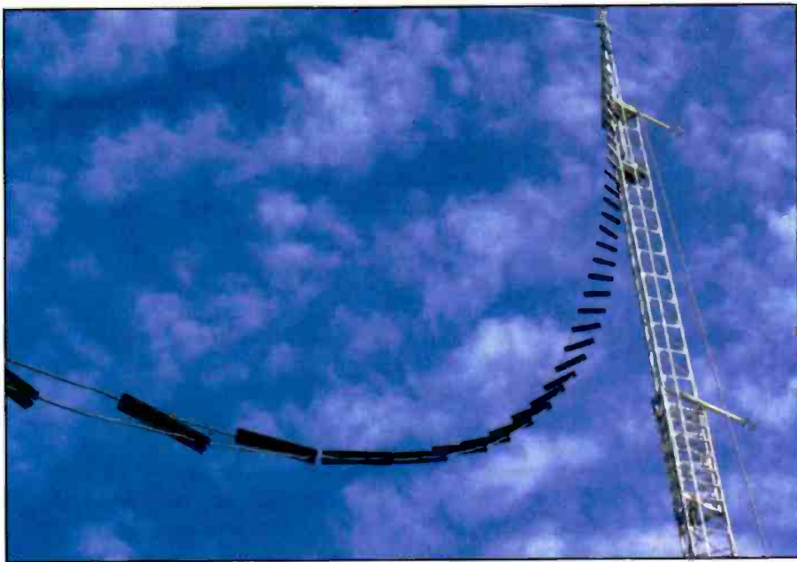
Photo A. Making your own 600-ohm open-wire line can be fun and educational—but it can also be tedious and frustrating! W7FG (see www.w7fg.net/ ) makes high-quality open-wire line and sells it for reasonable prices. When I moved, I uninstalled my big loop, which was fed with W7FG line, thinking I'd replace the used line at my new QTH. Upon inspection, however, the existing line was in perfect shape, Minnesota winters and all. So, I haven't had the need to buy more!
