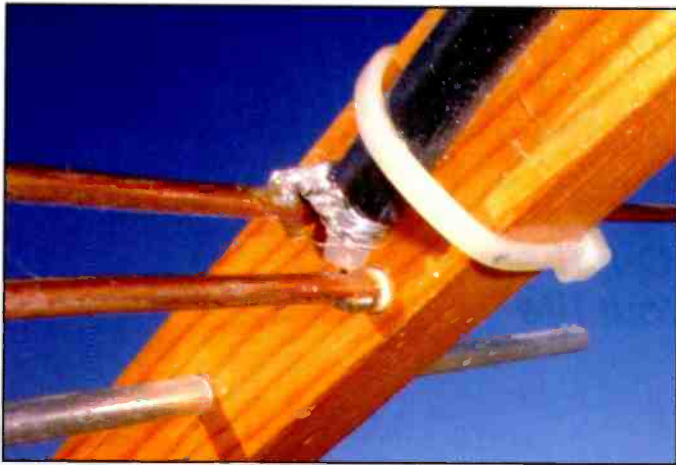
Photo C. Attaching the coax to the driven element.
