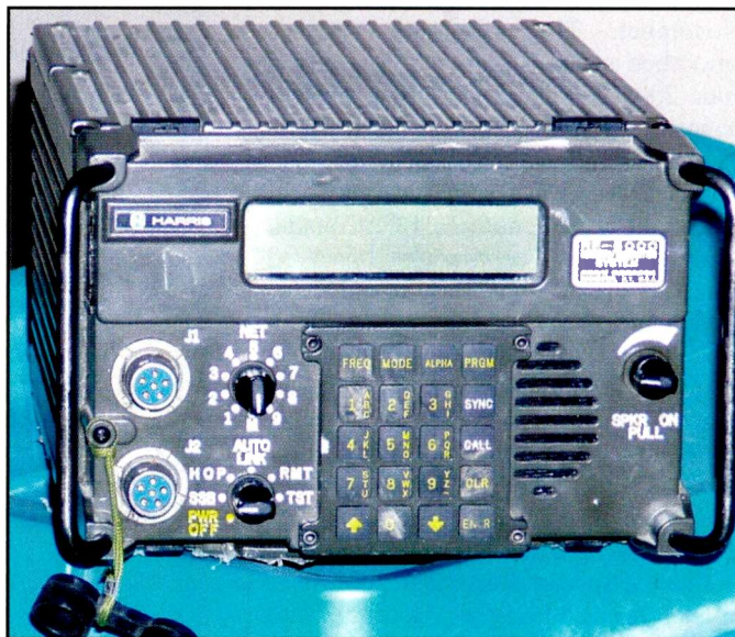
Photo A. The Harris RF-5000 series of DSP radios from the late 1980s represented the pioneering era of software-defined radio (SDR). This is the RF-5020, which as you can see was built tough and represented a real departure from earlier military design by incorporating LCD display and push button operation.
