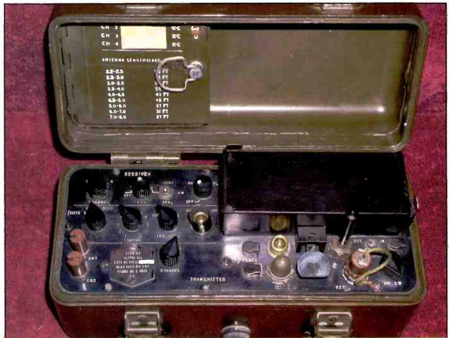
The AN/PRC-64 was the CIA’s choice for a small, clandestine HF CW rig during the Vietnam era. Made by Delco, the PRC-64/Delco 5300 covered 2.2 to 6 MHz and 3 to 8 MHz, respectively. It can receive AM/SSB/CW and transmit AM phone and CW. Power output is 5 watts on CW and 1.5 watts on AM phone. This unit, like the TRC-77(A) and GRC-109, can be interfaced with the GRA-71 code burst transmission unit to transmit messages at 300 wpm! This unit was all solid-state and weighed in at 5 pounds. The radio was a four-channel crystal-controlled rig that served with CIA operatives as well as U.S. Special Forces.
