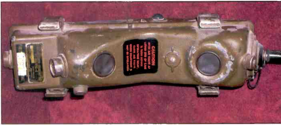
The AN/PRC-6 replaced the BC-611 just prior to the start of the Korean War. The Prick-Six was a wideband FM handheld radio that used pencil tubes and a high-voltage battery to produce a whopping 250 mW of RF power. The frequency range was low-band VHF, which means you can convert one of these handhelds to work on 6 meters (51.0 MHz) in fine style. Range is around one mile.
