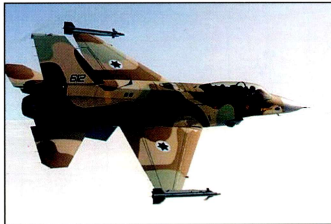
The F-161 looks radically different from other F-16s, with conformal fuel tanks, dorsal spine, and numerous fairings and bulges for undisclosed equipment.
