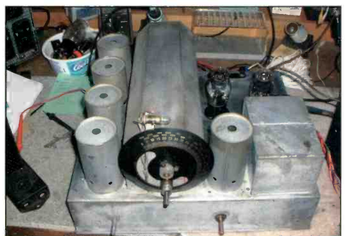
Photo D. The heart of the Majestic 90 is this seven-tube TRF radio receiver. The operating voltages were supplied by the outboard 9P6 power pack shown in Photo A.
