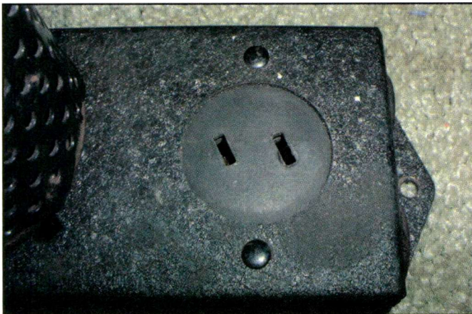
Photo E. A special 25-degree socket was used for the AC plug going to the 9P6 power pack. It allowed the 9P6 to be easily removed for servicing, and also prevented the 9P6 from being directly plugged into a power outlet.
