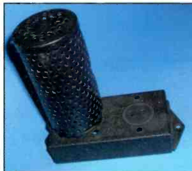
Photo B. Majestic included the 9P6 ballast regulator to accommodate a wide range of AC line voltages between 100 and 130 VAC, as might have been encountered during the 1920s.
