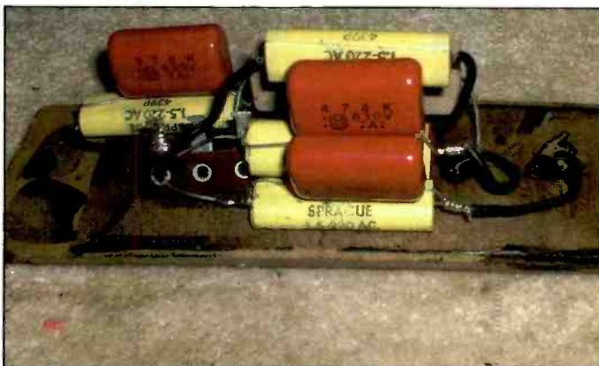
Photo L. The encapsulated block of paper filter capacitors was replaced with these tiny Mylar equivalents. Mylar capacitors will provide a much longer service life compared to electrolytic filter capacitors. Note that the original 2000-ohm filter choke (part of the encapsulated package) was replaced with a 2000-ohm resistor 10-watt wire wound resistor.
