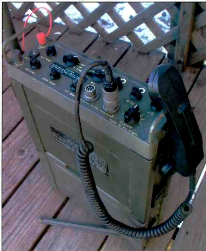
The AN/PRC-74 is a great HF man-pack radio that can be procured for around $500 on e-Bay or at swap meets. This unit is a synthesized solid-state HF transceiver capable of transmitting and receiving USB voice from 2 to 12 MHz (PRC-77(A)) and 2 to 18 MHz (PRC-77(B & C)). This Vietnam-era radio and was the world's first synthesized HF packset. Power requirements are 10-17 VDC; it weighs in at 24 pounds.
