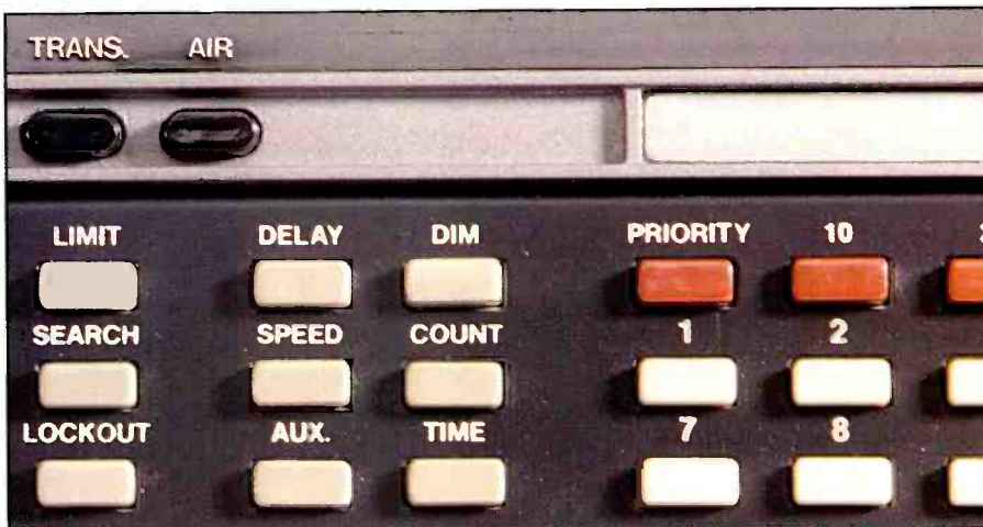
Aviation scanning has been featured on most scanner models since the early days of programmable scanners. This early Bearcat had "service search," a one-touch feature to scan the entire air band. It was a good way to find frequencies if you didn't know what was around.
